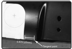
**9.** Locate the hood latch indentation outer tangent point and measure 0.875" left of tangent to locate supplied cutting template.
