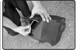
**3.** Use an allen wrench and remove the Air Box Shield Air Director from the Injen air box. This shield will no longer be used when installing the Injen EVO15069 Scoop
