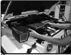
**6.** Once the Injen air scoop is assembled onto the Injen air box, re-installed the Injen air box and re-connect the intake tube and 4.0" hump hose from figure 2
