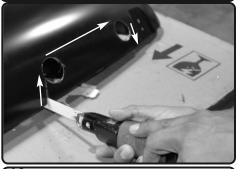
**12.** The line drawn from the template in figure 10 will be a guide to cut using an air saw to cut a straight line.
