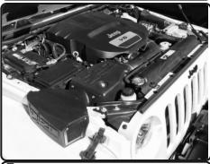
**7.** Injen intake system and air scoop installed.
