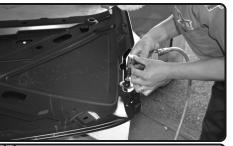
**14.** Use a flat grinder to straighten the edges and clean up all the metal burrs. Slowly grind back on the open. Only grind what you need for additional clearance. Please use caution and have proper safety equipement like goggles and air respirator!!!
