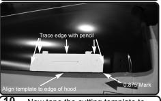
**10.** Now tape the cutting template to the hood from the 0.875" mark from figure 9 and make sure you line up the bottom of the cutting template to the edge of the hood. Use a pencil and trace the edge of the template for a cutting guide for the next step.
