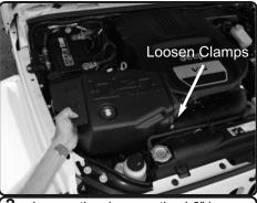
**2.** Loosen the clamp on the 4.0" hump hose and remove the Injen intake box from the engine bay.
