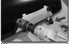
**11.** Using the crosshairs on the cutting template as a guide, use a 1 3/4" hole saw and drill out the two holes on the template. Make sure you drill past the second layer of the hood. *Please use caution!!!*
