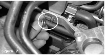
Once the intake has been aligned to the threaded stud continue to screw the nut back onto the stud, tighten the nut just enough to hold the intake in place.
