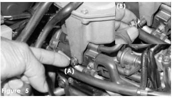
Remove this m6 nut where the bracket on the intake will be located(A). Once the nut has been removed continue to align the assembled intake in place(B).
