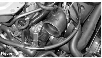
The stock air intake box and air intake duct has been removed from the engine compartment.
