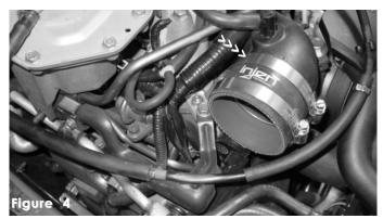
Press the 2 7/8" straight hose over the throttle body and use two clamps but only tighten the clamp on the throttle body.
