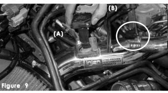
Insert the mass air flow sensor into the machined adapter on the intake(A). Press the sensor in until it bottoms out then use the stock screws to fasten the sensor in place(B).
