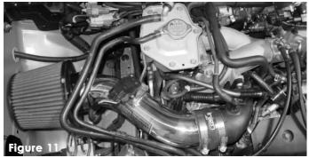
Press the harness clip into the mass air flow sensor until you hear it snap firmly in place.
