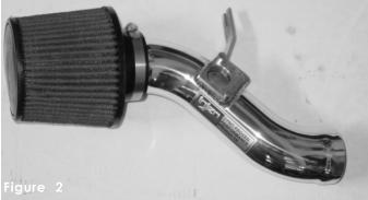
Take the short ram intake system and air filter and assemble them together. Press the filter over the 3" side of the intake and tighten the clamp on the filter neck.
