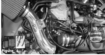
Take the assembled short ram intake system and position it in place. The 2 7/8' end should fit snugly into the hose on the throttle body.
