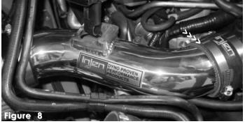
Insert the 2  $7/8^{\circ}$  end on the intake into the hose on the throttle body. Semi-tighten the clamp on the hose to hold the intake in place.
