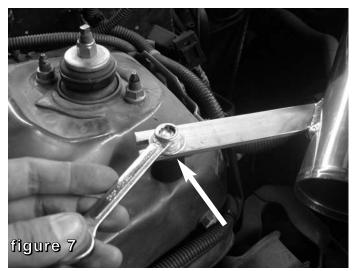
Secure the bracket using the washer and nut provided. Tighten using 10mm socket or wrench.
