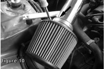
Install the filter to the tube and tighten using 8mm nut driver. Your installation is now complete. Thank you for choosing Injen.
