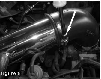
Position best fit and tighten the clamps on the elbow using 8mm nut driver.
