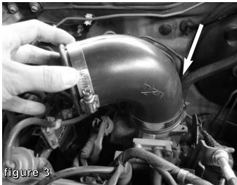
Install the elbow hose to the throttle body and secure using the 2 #48 clamps provided.
