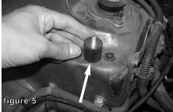
Install the vibra mount to the thredded insert located on the strut tower. Secure and tighten.
