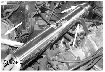
Install the intake tube position to elbow and bracket to the vibra mount. Connect the crank case line to the fitting on the intake tube.
