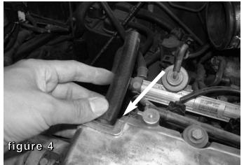
Attach to the engine crank case fitting the provided 10mm hose.
