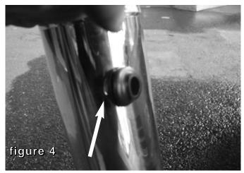
Install the grommet to the 3/4" hole on the intake tube.
