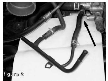
Remove the factory intake system out of vehicle. Remove the crank case/coolant throttle body hard line out of vehicle and replace with new 12" Length 6mm hose provided.
