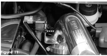
Insert the vacuum switching valve over the mounting bracket. Use the zip tie provided in this kit to keep the vacuum switching valve from vibrating.
