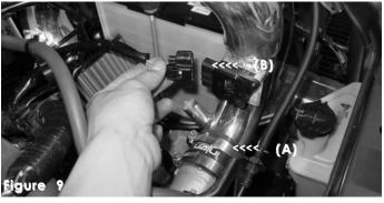
The intake is positioned in place at the throttle body (A) and the clamp is semi-tightened for support. Take the harness clip and press it into the air temperature sensor until you hear a quick snap (B).
