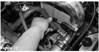
Press the end of the 15mm hose over the 5/8" port on the intake, use the stock hose clamp to secure the hose in place.
