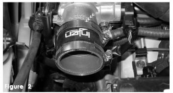
Press the 2 1/4" straight hose over the throttle body and use two clamps, tighten the clamp on the throttle body at this point.
