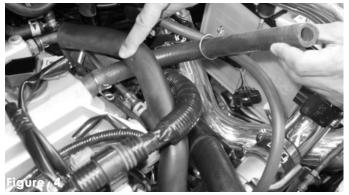
Take the 14" 15mm heater hose and press it over the port located on the crankcase. The stock hose clamps will be used to prevent the hose from slipping out.
