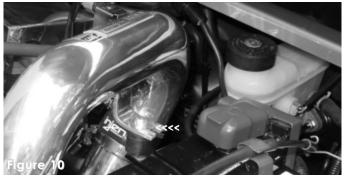
Line up the bracket on the intake to the vibra-mount stud and use an m6 flange nut and fender washer to secure the intake in place.
