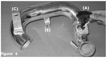
The air temperature sensor is removed from the stock air box and inserted into the machined adapter, the stock screws are used to fasten the sensor in place(A). The short L-bracket in the middle of the intake will be aligned to the vibra-mount stud (B). The long bracket is the mounting bracket for the vacuum switching valve.
