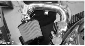
The filter is now pressed onto the end of the intake and the clamp on the filter neck is fastened tight.
