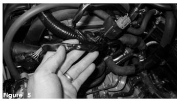
The harness line is moved out of the way prior to installing the primary intake. The harness will be used later in the instructions to reconnect the air temperature sensor
