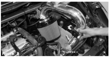
Lower the assembled intake system into the engine compartment and press the 2 1/4" end into the hose on the throttle body.
