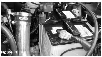
Take the male/female vibra-mount and screw it on the end of the threaded battery post. The vibra-mount will need to be adjusted up or down according to the bracket location on the primary intake.
