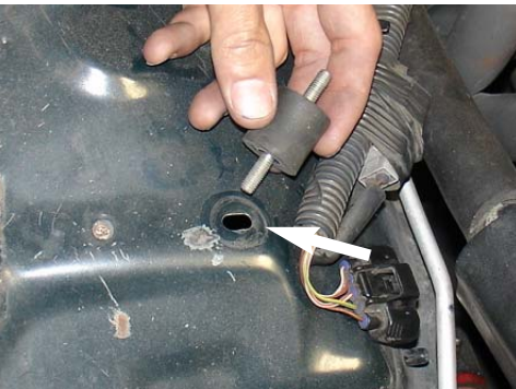
Insert vibra-mount into the pre-drill hole located on the fender well.
