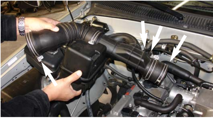
Loosen the clamps on the air intake box and the throttle body, remove the two vacuum lines connected to the intake and then continue to remove the air intake duct as shown above.
