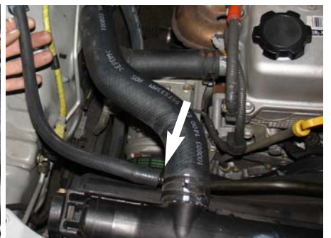
The 14"-10mm vacuum hose is now connected to the charcoal canister hard pipe.
