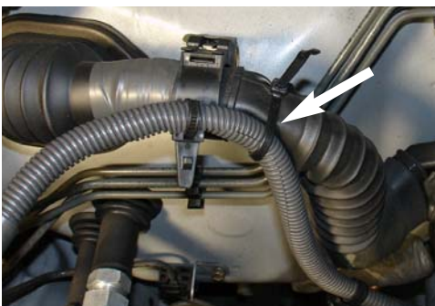
Use the zip tie to secure the sensor harness to the ECU main harness as shown above.
