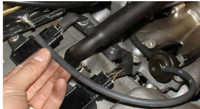
The stock 4mm pressure fuel regulator line is now pressed onto the 3/16" intake port.
