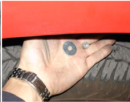
Go underneath the fender well, take the m6 flange nut and fender washer and secure the vibra-mount to the fender well.
