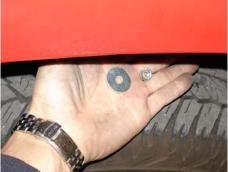
Go underneath the fender well, take the m6 flange nut and fender washer and secure the vibra-mount to the fender well.
