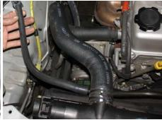
The 14"-10mm vacuum hose is now connected to the charcoal canister hard pipe.
