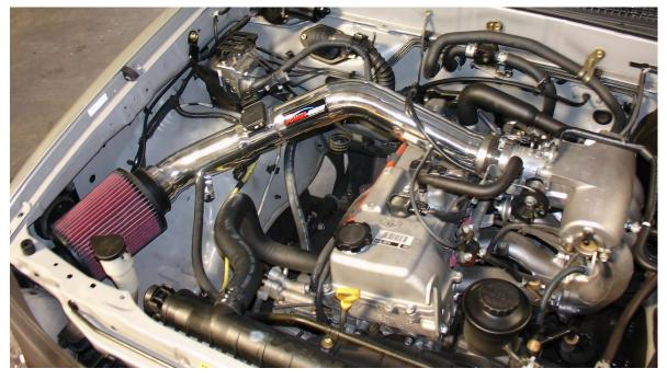
You have purchased the Worlds first tuned intake system available anywhere. The Power-Flow intake system features Injen's patent pending MR Technology used to tune the intake. With Power-Flow, calibrating of the MAF sensor is not required because the intake system comes tuned for use. Use only Injen replacement filters. The use of any other filter will change the air/fuel ratio that can cause damage to your engine.
