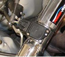
Take the harness clip and press it over the mass air flow sensor until you hear it snap in place, this will assure a good connection.
