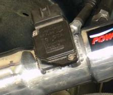
Once the mass air flow sensor has been firmly inserted into the machined sensor adapter continue to use the stock screws to fasten the sensor to the adapter
