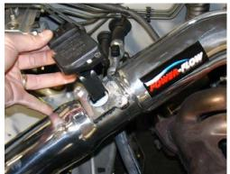
Take the mass air flow sensor and carefully insert it into the machined sensor adapter. we recommend you use a dab of light oil of water to wet the O-ring. This will allow the O-ring to slip into the hole for a better seal.
