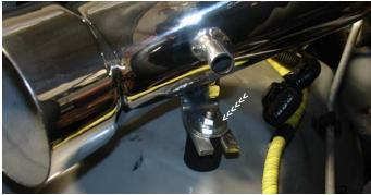
The flange nut and fender washer is screwed onto the vibra-mount stud. Do not over- tighten the flange nut at this point until the filter has been placed on the
