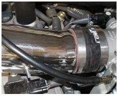
The intake is inserted into the throttle body hose and the intake bracket is lined up to the vibra-mount stud.
