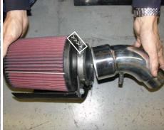
Press the 3 1/2" filter neck over the secondary intake as shown above. Once the intake has butted up against the filter neck stops continue to tighten the clamp. The Power-heat shield shown on the filter is an accessory not included in this kit.
