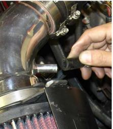
Once the 3/8" coupler and 6"-10mm hose have been installed continue to connect or press the hose over the 1/2" intake port as shown above.
