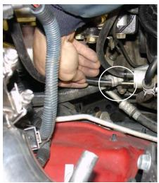
The other end of the 18" -6mm vacuum hose is pressed over the power-steering switch port as shown above.
