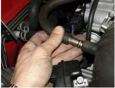
Pull the CC breather line from the air intake duct located by the passenger side firewall. The 13" 10mm vacuum line will be used once the intake has been installed.
