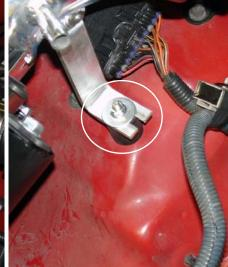
The 2 1/2" end on the secondary intake is lined up to the Once the secondary intake has been pressed into the 2 1/2" straight hose the intake bracket is secured using the m6 flange nut and fender washer.
