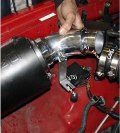
hose located on the mass air flow sensor (A) . The intake
