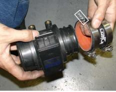
Press the 2 1/2" straight hose over the inlet side of the mass air flow sensor. Use to two Power-clamps and tighten the clamp on the mass air flow sensor end.
