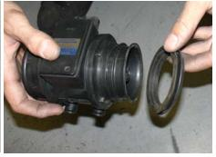
The sealing grommet has been removed and set aside. This grommet will not be needed to complete the installation.
