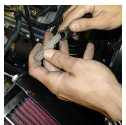
The 6" 10mm hose is pressed over the 3/8" coupler from that leads over to the Evap charcoal canister. This line is used to extend the line to allow for slack.
