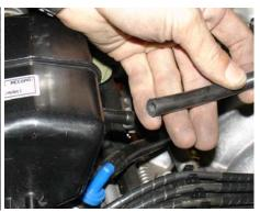
Remove the 6mm stock hose connected to the air intake resonator box. This hose leads to the fuel pressure regulator below the throttle body.
