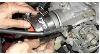
Press the 2 3/4" straight hose over the throttle body and use two power clamps on the straight hose, tighten the clamp located over the throttle body.
