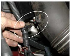
Disconnect the harness clip held on to the lower air intake duct.
