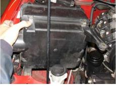
Remove the m6 bolts that secures the air intake box to the wheel well. Once all bolts have been removed continue to remove the entire air intake box from the engine compartment.
