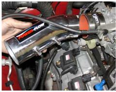
Take the primary intake and press the 2 3/4" end into the straight hose located on the throttle body. Semitighten the clamp just enough to hold the primary intake in place.
