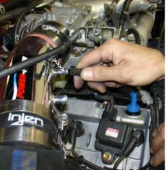
The hose just pressed over the fuel regulator port is connected to the first 3/8" port located on the primary intake.
