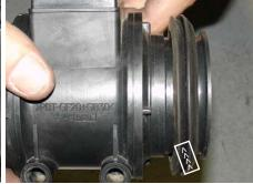
Remove the sealing grommet from the air mass sensor located on the inlet side of the sensor.
