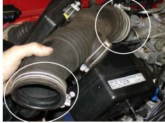
Loosen the two clamp located on each side of the air intake duct. Once the clamps have been loosened removed the entire air intake duct from the throttle body and air intake box.
