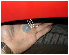
Reach underneath the wheel well and use the m6 flange nut and washer to secure the vibra-mount in place.
