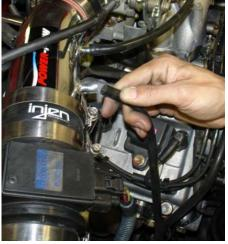
The 18"-6mm vacuum hose is pressed over the second intake port located on the primary intake. The other end lead down to the to Power steering switch port.
