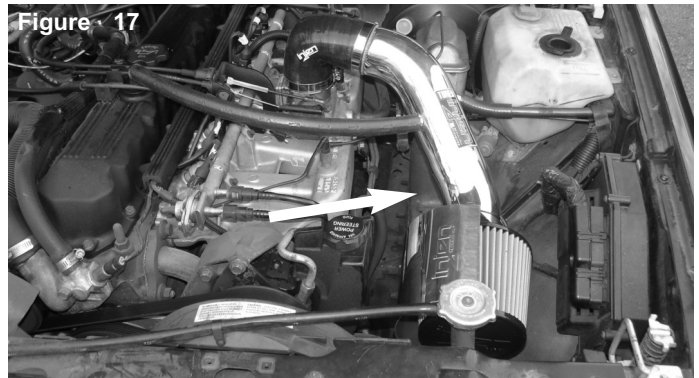
Position the intake so that it does not hit any lines or comes close to anything. Your Injen intake installation is now complete. Check for any rubbing or any rattling. Tighten all clamps and re-tighten if necessary.
