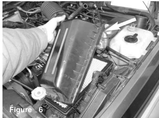
Figure 6 Lift up and pull the upper half of the air box assembly.
