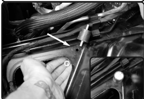
8. Install the vibramount to the hole on the frame. Use the M6 nut and secure.
