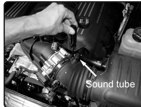
3. Loosen the clamp on throttle body using 8mm nut driver.
