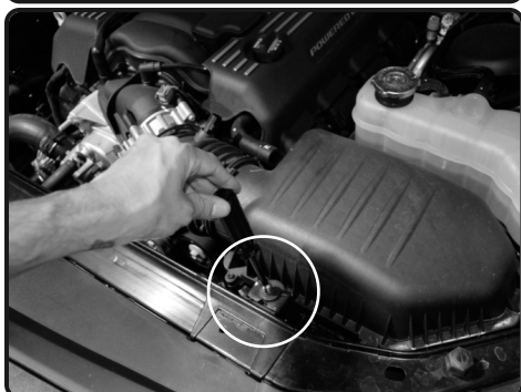
4. Loosen the bolt holding in the airbox using 8mm nut driver.
