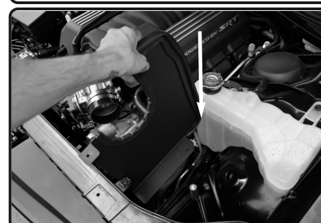
11. Now install the heatshield into the vehicle and position.
