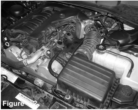
Complete stock air intake cleaner and air intake duct.
