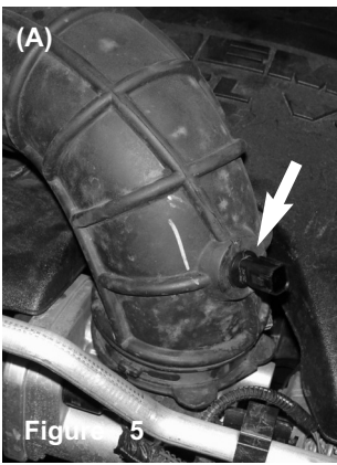
Figure 6(A) Air temp sensor with harness removed Figure 6(B) Firmly pull air temp sensor out of factory air duct. This sensor will be re-used later.
