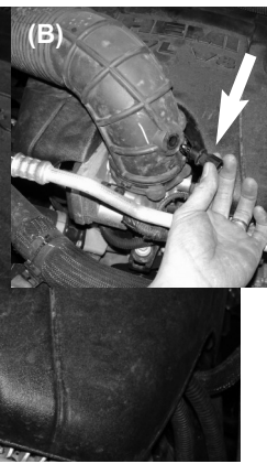
Figure 6(A) Air temp sensor with harness removed Figure 6(B) Firmly pull air temp sensor out of factory air duct. This sensor will be re-used later.
