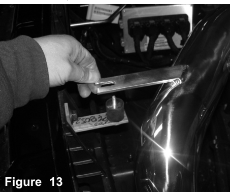
Figure 14 Align the bracket onto the vibramount
