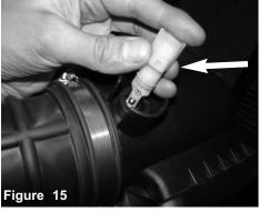
Twist and remove the temp sensor from the air box.
