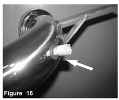
Install the temp sensor to the grommet and secure.
