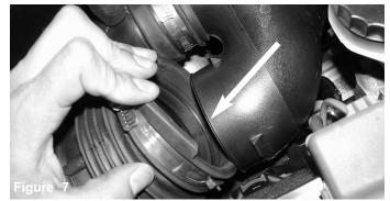
Pull back the intake tube from the "Y" split.
