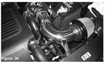
Congratulations! You have just completed the installation of this intake system. Periodically, check the alignment of the intake, normal wear and tear can cause nuts and bolts to come loose. <u>Note: Check clearance and adjust if needed!</u> <u>Failure to check the alignment and adjust the intake can cause damage</u> that will void the warranty. Injen Technology is not responsible for any damages caused by/from improper installation.
