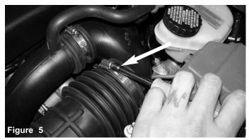
Loosen the intake tube clamp using 8mm nut driver.
