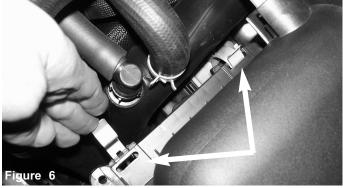
Un-clip the 2 clips holding in the upper half of the air box.
