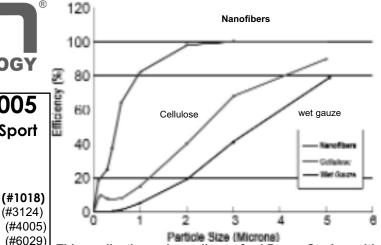
Nanofiber technology: Is an oil free filtration media that has been used exclusively in heavy duty applications, including the US Army's Abrams M1 tanks. Injen's is now making it available to diesel applications and vary soon will be available for the gas auto/light truck market
