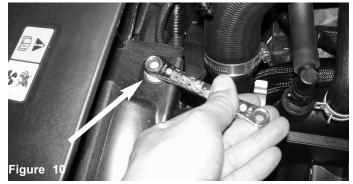
Locate the screw on the radiator support next to the air box. Loosen using 10mm wrench.
