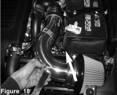
Install the intake assembly into the vehicle and position to throttle body and bracket to vibra mount.
