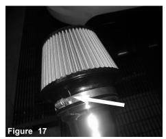
Install the filter to the intake tube and tighten using 8mm nut driver.
