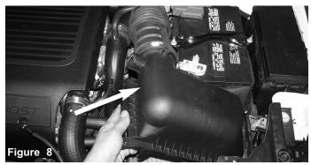
Now lift up and remove the stock upper intake assembly out of the vehicle.
