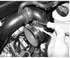
Install the step hose with clamps provided to the "Y" split. Tighten the clamp on the "Y" split only.
