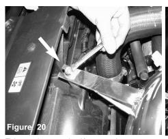
Tighten and secure using 10mm wrench.
