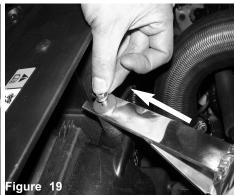
Secure the bracket using provided Fender washer and M6 nut.
