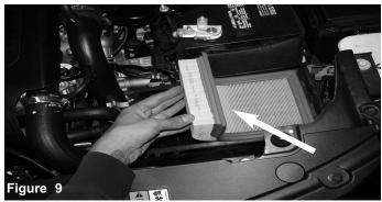
Remove the stock filter out of the vehicle.
