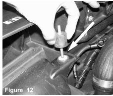
Replace using provided M6 long stud. Secure using the long stud side and tighten.
