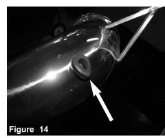
Now install the rubber grommet to the hole on the intake tube.
