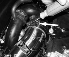
TIghten the clamp on the intake tube using 8mm nut driver.
