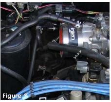
Place the 3" (76mm) straight hose over the throttle body. Place two clamps on the 3" hose and tighten the clamp on the throttle body end.
