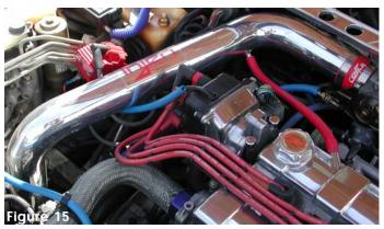
Align the entire intake for best possible fit. Once the intake has been cleared from any moving parts or free from contact with engine parts, continue to tighten all nuts. bolts and clamps.
