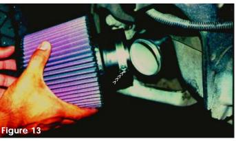
The filter neck is aligned and pressed over the the end of the intake. Once the intake has reached the the desired stops inside of the filter, continue to tighten the filter neck clamp.
