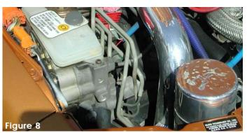
The filter end side of the intake is lowered into the engine compartment. The lower end of the intake is wedged between the engine and the frame as shown above. The intake bracket is also aligned to the vibra-mount stud.
