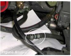
Once both coolant lines have been joined together with the coupler, continue to use the stock clamps to secure the in place.
