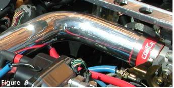
Once the intake bracket has been aligned to the vibra-mount stud, the top end of the intake is pressed into the throttle body hose. The power band on the intake side is semi-tightened to secure the intake in place.
