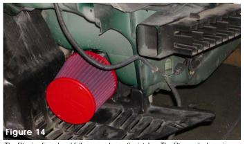
The filter is aligned and fully pressed over the intake. The filter neck clamp is also fastened to prevent the filter from falling off.
