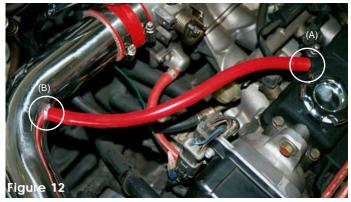
Press the 13"-10mm hose over the crankcase port (A) press the other end over the 1/2" intake port (B).
