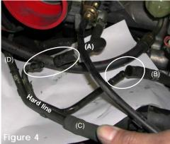
Remove the PCV hard pipe connecting the coolant line(A) and (B) and breather hose (C) and (D). Coolant lines are disconnected (A) and and joined together with the 1/4" coupler.
