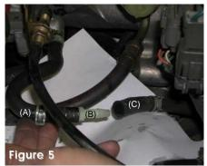
Once the PCV hard pipe has been removed, insert 1/4" coupler (B) into the intake coolant port (A). Insert coupler into the coolant delivery port (C). U
