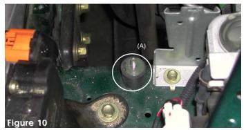
Once the top intake has been pressed into the throttle body hose, the intake bracket is aligned to the vibra-mount stud. Use the fender washer and flange nut to secure the intake in place (A).
