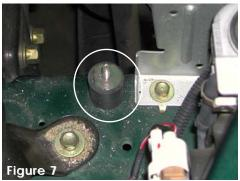
The vibra-mount is screwed into the passenger side frame next to the reservoir bottle brace.
