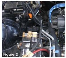
Loosen clamps on the air box and throttle body. Unhitch tension clips on the air box lid. Remove the top lid and remove panel filter. Unscrew bolts on the lower air box cleaner, then pull lower box cleaner out. The resonator box will also be pulled out.
