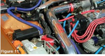
The entire cold air intake has been installed and aligned to all mounting points. Good clearance is a must through out the length of the intake. Periodic refitting will be required to adjust for possible moving of the intake, clamps or vacuum lines
