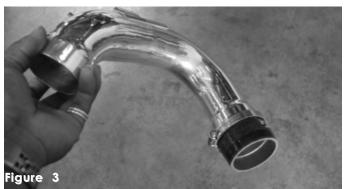
Slip the remaining 2 3/4" straight hose over the end of the Primary intake. The side opposite of the machined adapter and vacuum port is the end where the hose will be placed, use a clamp to fasten the hose to the intake.
