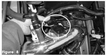
Once the mass air flow sensor has been fastened reconnect the harness clip to the sensor until you hear it snap.
