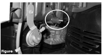
Screw the vibra-mount into the bracket located on the side frame. Note: The bumper will have to be removed in order to install the vibra-mount and secondary intake.
