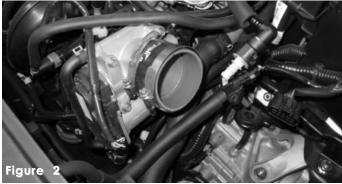
Press the 2 3/4" straight hose over the throttle body. Use two clamps on the 2 3/4" hose but only tighten the clamp on the throttle body.
