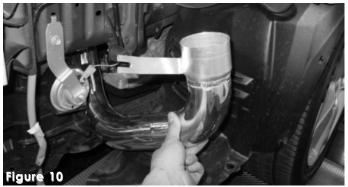
Take the secondary intake and insert the top end into the engine compartment by way of the bumper opening. The bracket on the intake will be facing outward.
