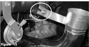
The bracket on the end of the secondary intake is lined up to the vibra-mount stud.
