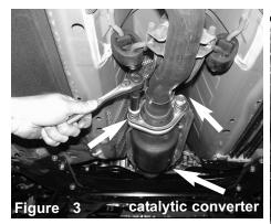
Use a 14mm socket and rachet and remove the two factory spring bolts connecting the exhaust system to the catalytic converter
