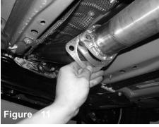
Place the supplied 3.00" gasket in between the Injen down pipe and exhaust system.
