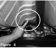
Due to the tight clearances and Injens down pipe design to minimize bends, it may require you to push up on the heat shield for added clearance indicated in the photo
