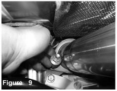
Re-use the factory spring bolts to reattach the Injen down pipe to the primary catalytic converter
