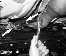
Add a long extension and swivel to the 14mm socket and rachet and loosen the two spring bolts that attaches the secondary cat to the primary cat.
