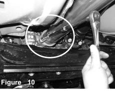
Use the 14mm socket, rachet, swivel and extension to tighten the spring bolts
