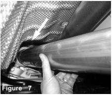
Attach the Injen secondary Cat-delete down pipe to the factory primary Cat. Make sure the top of the down pipe does not come into contact with the heat-shield indicated by the arrow.
