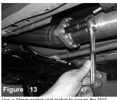
Use a 14mm socket and rachet to secure the M10 nuts and bolts to the flanges
