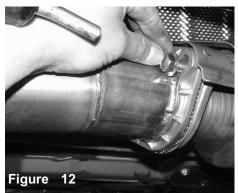
Place two supplied M10 nuts and bolts attaching the Injen down pipe to the exhaust system
