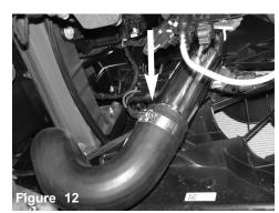
Secure the bottom of the intercooler piping and tighten using 8mm nut driver.
