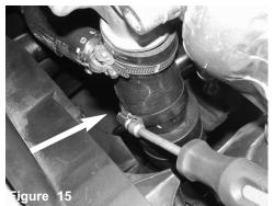
With pliers, break or cut the factory 1 time use clamps. Remove and pull back the hose.
