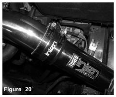
Once connected, position for the best fit. Secure the bracket using provided m6 nut and fender washer.
