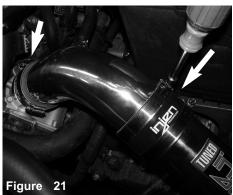
Tighten all clamps using 8mm nut driver.
