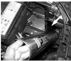
Place the Long Injen intake pipe through the opening under the drivers side headlight and position to the hose and the bracket to the vibra mount.
