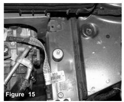
Position the vibra mount like image above and tighten.
