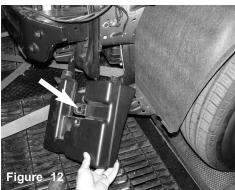
Locate the air box resonator in the drivers side front bumper wheel well area. Remove the 10mm bolt attaching the resonator to the chassis and then pull the entire air box resonator out.
