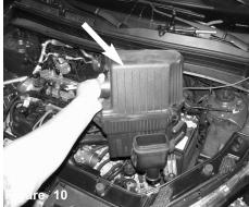
Lift up on the air box assembly and remove the entire air box assembly from the engine bay.
