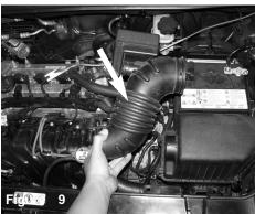
disconnect the air duct from the throttle body and air box and remove the air duct hose
