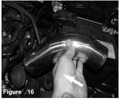
Place the short injen intake pipe onto the throttle body hose. *Make sure longer side of tube is on throttle body*.
