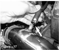
Position the crank case line to the fitting on the intake tube. Secure using the factory clamp.
