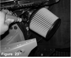
Place the filter onto the end of the intake pipe. Tighten the clamp on the filter with a 8mm nut driver to secure the filter to the intake pipe.
