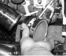
Place the 2.75" straight hose with clamps provided to the hose and secure on the tube only.
