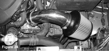
Your intake installation is now complete. Go over all your clamps and fittings to make sure they are snug. Check the clearance on the pipe and make sure it does not make contact with any components in the engine bay. Note: For extreme weather conditions, remove lower intake assembly, and place filter on upper intake tube for short ram install.
