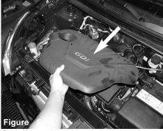
Firmly lift up on the engine cover and remove the engine cover from the engine bay for now. This cover will be re-installed later
