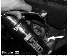
You may down tighten the M6 nut to secure the intake bracket to the vibra mount
