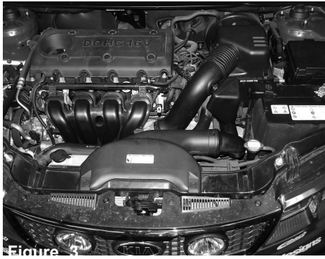
Figure 3 Stock air box cleaner and air ducts shown in this picture. Before getting started with the installation, be sure to disconnect the negative battery terminal.
