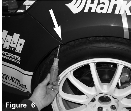
Figure 6 Unscrew and removed the 8mm screw under the passanger and driver side wheel well.
