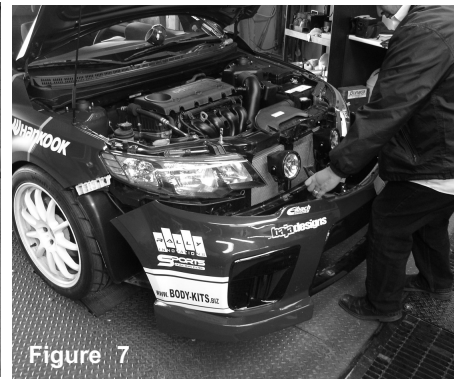
Figure 7 Once all plastic clips and screws have been removed continue to pull the front bumper off
