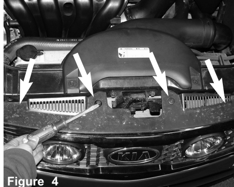
Figure 4 Loosen and remove the four plastic clips from the front shroud cover.
