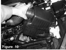
Now carefully lift up and remove the complete air box Install the new 8mm hose to the crank case fitting. assembly from the vehicle.
