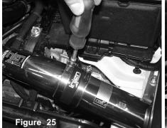
Tighten all clamps using 8mm nut driver.
