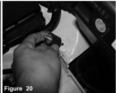
Carefully pull back the fog lamp harness from resonator Install the vibra mount to the factory thredded fitting where the air box mounted to. Secure and tighten.
