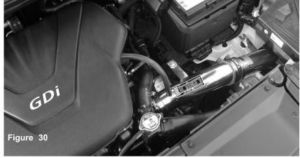
Congratulations! You have just completed the installation of this intake system. Periodically, check the alignment of the intake, normal wear and tear can cause nuts and bolts to come loose. Failure to check the alignment and adjust the intake can cause damage that will void the warranty.
