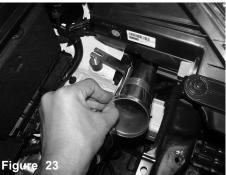
Install the lower intake assembly. Position for the best possible fit.
