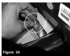
Position for the best possible fit. Secure the bracket using provided M6 nut and washer.
