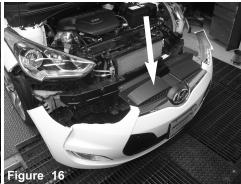
Removal of the front bumper cover is necessary for the CAI install. remove the 4 screws on radiator support and remaining plasitic push-clips using phillips screwdriver both on top and under the cover. Disconnect Fog lamps.
