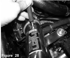
Attach the crank case hose to the fitting on the intake tube and secure. Re-install the front bumper cover and re-connect the battery.
