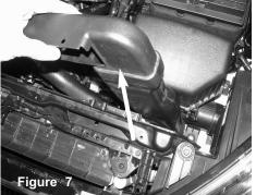
Push the clips holding in the factory scoop. Pull out and remove the facotry scoop.
