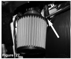
Install the filter and tighten using 8mm nut driver.
