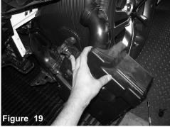
and any other lines, now slide resonator out and remove.
