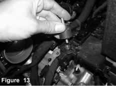
Install the vibra mount to the factory thredded fitting where the air box mounted to. Secure and tighten.
