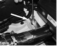
Tighten bracket using 10mm socket and ratchet.
