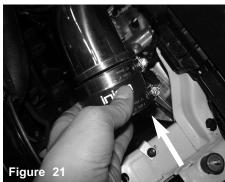
Install the straight hose with clamps provided to the upper intake assembly.
