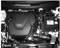
Removal of the lower intake assembly and install the filter to the uppwer intake assembly for the Short Ram intake system.
