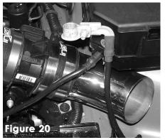
The secondary intake is now installed facing to the front of the car.
