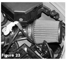
The filter is now pressed over the intake end and the filter neck clamp is tightened
