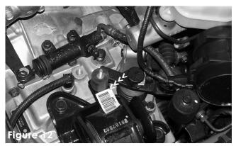
Turn vibra-mount until it is sitting flush with the engine mount brace.
