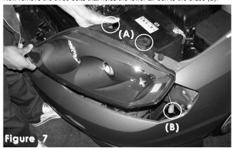
Remove two bolts located on the head lamp frame (A). Disconnect harness clip from the rear head lamp and remove harness clip (B). Once bolts and clips have been removed, continue to remove head lamp as shown above.
