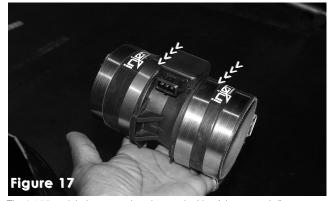
The 3 1/8" straight hose are placed on each side of the mass air flow sensor, two power bands are used on each side of the sensor. Tighten the two clamps to the center of the mass air flow sensor for now.
