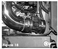
Lower the mass air flow sensor into the engine compartment and press it over the end of the intake as shown above.
