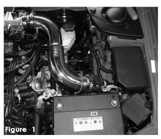
Hydro-Shield used for this application X-1033
