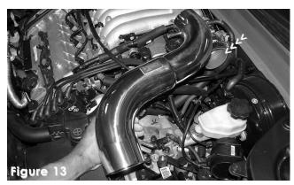
Lower the primary intake into the engine compartment and align it to the throttle body hose.
