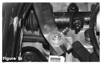
The m6 flange nut and fender are used to secure the intake bracket to the vibra-mount stud.
