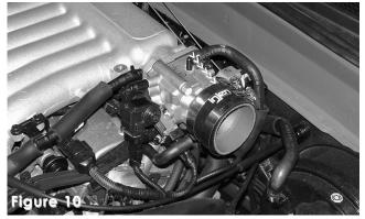
Press the 2 3/4" straight hose over the throttle body and use two power bands, tighten the clamp on the throttle body.
