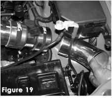
The secondary intake is then lined up the mass air flow sensor and inserted into the hose.
