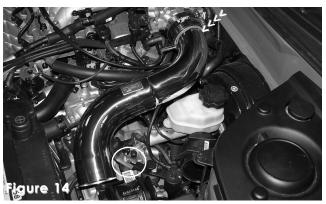
Insert primary intake into the throttle body hose while aligning the intake bracket to the vibra-mount stud.
