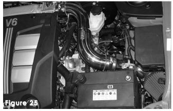
Align the entire intake for the best possible fit. Once you have position the intake to prevent any rubbing or rattling, continue to tighten all nuts, bolts and clamps.
