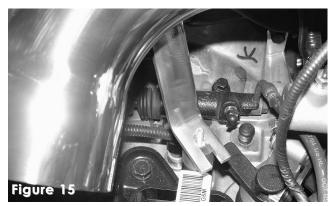
The intake bracket should sit even and flush with the vibramount stud as shown above
