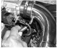
The stock air vacuum hose is lined up and pressed over the 3/16" intake port.
