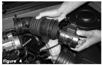
Once you have remove the entire air intake duct, continue to loosen clamp on the plastic air duct from the inlet side. Continue to pull the mass air flow sensor from the air intake duct.
