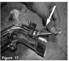
Now install the temp sensor into the new intake tube. secure using provided M6 screw.
