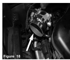
Install the straight hose with clamps to the throttle body and tighten the clamp on the throttle body only.
