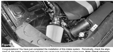
Congratulations! You have just completed the installation of this intake system. Periodically, check the alignment of the intake, normal wear and tear can cause nuts and bolts to come loose. <u>Note: Check clearance</u> <u>and adjust if needed! Failure to check the alignment and adjust the intake can cause damage that will</u> <u>void the warranty. Injen Technology is not responsible for any damages caused by/from improper</u> <u>installation.</u>
