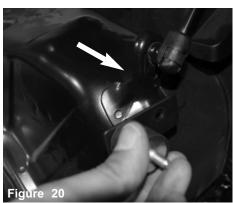
Locate the hood strut on top of the front suspension strut tower.locate the hole on the hood strut bracket. make sure the offset hole on bracket is facing up.
