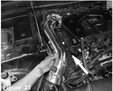
Install the intake tube and position the bracket to the vibra mount and to the throttle body.
