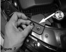
Remove the push clips holding in the stock airbox components and the factory scoop.
