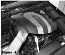
Lift up and remove the engine cover.
