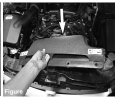
lift up and remove the factory scoop.
