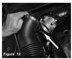
Loosen the clamp on the throttle body, pull back the intake tube.
