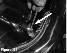
Secure the bracket to the vibramount assembly. Secure using provided M6 nut and fender washer.
