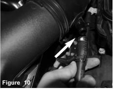
With pliers, remove the crankcase line.
