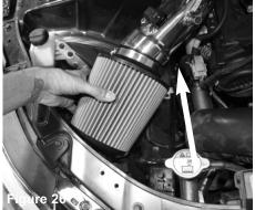
Install the air filter to the intake tube.
