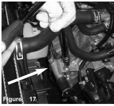
loosen the 13mm bolt on engine for the bracket on intake to be secured.
