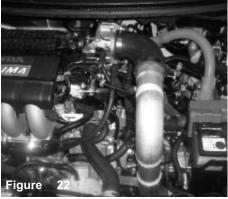
Tighten all the clamps on the intake tube using 8mm nut driver.
