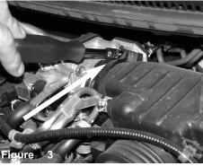
With 5.5mm socket, loosen the clamp on throttle body.
