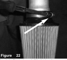
Attach the filter to the end of the intake tube.
