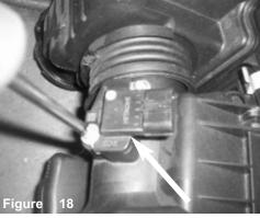
With phillips screwdriver, loosen the MAF sensor from the air box.
