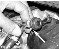
Carefully pull back the crank case linr away from air box.
