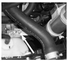
Secure the bracket on intake tube from step 17 and tighten.
