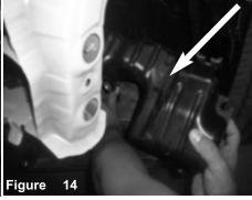
Carefuly pull out the air box resonator.
