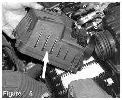
Un-clip the upper half of stock air box and lift and pull of vehicle. Remove stock air filter.
