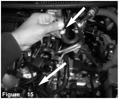
Remove the complete crank case/throttle body coolant assembly.
