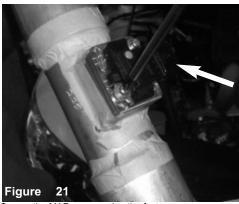
Secure the MAF sensor using the factory screws.
