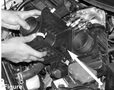
Carefully lift and remove the stock air box out of vehicle.
