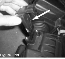
Remove the MAF sensor from the air box.
