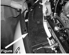
The front bumper cover needs to be removed to complete the rest of removal of stock air box. The front bumper contains push clips and screws. Loosen and remove all screws and clips.
