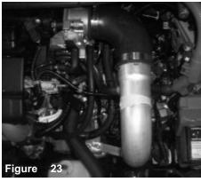
Align the entire intake for the best possible fit. Once you have rechecked and cleared the intake from all moving parts, continue to tighten all nuts, bolts and clamps
