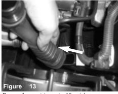
Remove the remaining parts of the air box.
