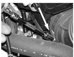
Loosen the rubber ram scoop from the air box and front of vehicle.
