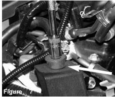
Loosen the screws holding the bottom half of air box using 10mm socket and ratchet.
