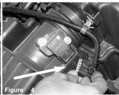
Disconnect the MAF sensor harness and pull back line away from air box.
