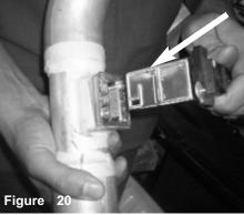
Install the MAF sensor into the new intake tube.
