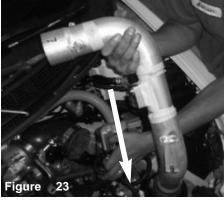
Install the elbow coupler with clamps to throttle body. Position the intake assembly into the vehicle.
