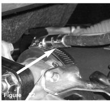
Tighten the clamps on the throttle body,
