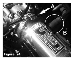
A)Position the intake tube for best fit and clearance. Tighten the clamps using 8mm nut driver. B) With provided 12mm hose, attach to fitting on intake tube to fitting on the crank case hard line.
