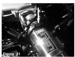
Position the intake tube to the throttle body. Do not tighten.
