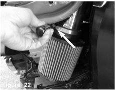
Install the filter to the intake tube and tighten using 8mm nut driver.
