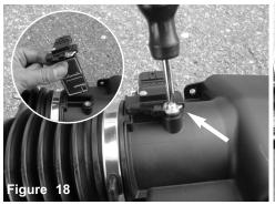
Loosen the 2 screws holding in the MAF sensor using phillips screwdriver and remove the sensor. Save the screws for later install.
