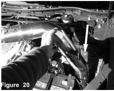
Now install the intake system into the vehicle and position to the throttle body and bracket to the vibra mount.
