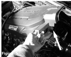
Lift up and remove the engine cover from the vehicle.
