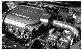
Align the entire intake for best possible fit. Once you have aligned and made sure that the length of the intake is free from any moving parts, continue to tighten all nuts, bolts and clamps.
