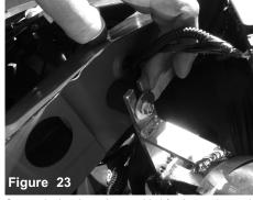
Secure the bracket using provided fender washer and M6 nut, positon for best fit and clearance and tighten using 10mm wrench.
