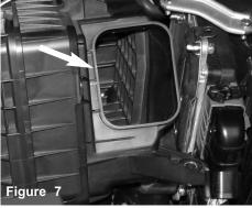
The air scoop is dislodged and pulled from the opening of the air box cleaner as shown above.
