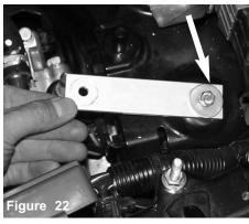
The extension bracket is placed over the pre-threaded hole that once held the air box cleaner in place. An m6 bolt and washer is used to fasten the bracket in place.
