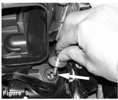
Once you have loosened the m6 bolt, continue to pull the m6 bolt out.
