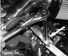
The fitment is checked again prior to tightening the m6 flange nut on the intake bracket and vibra-mount.
