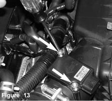
An allen screwdriver is used to loosen the two stock screws from the mass air flow sensor.
