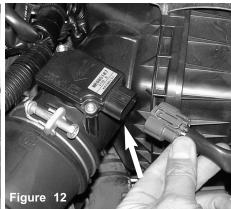
Depress the clip on top of the harness and pull the harness away from the mass air flow sensor.
