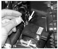
The two mass air flow sensor screws are loosened and removed in order to pull the sensor out of the sensor housing.
