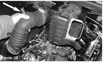
The stock air intake box and air intake duct is now pulled out of the engine compartment.
