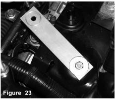
The extension bracket is now in place, semi-tighten the clamp for now.
