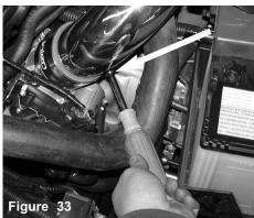
Once you have aligned the intake continue to tighten the hose clamp located over the intake,
