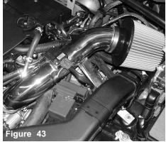
Check the entire intake system for best possible fit. Make sure there are no rubbing parts, rattles, or vacuum leaks, then continue to tighten all nuts, bolts and
