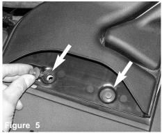
Once you have loosened the plastic clips, continue to pull up on the clips as shown above.
