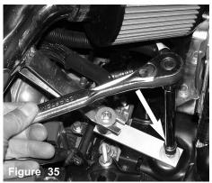
The m6 nut is now tightened over the extension bracket
