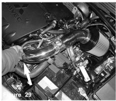
The assembled filter and intake is now lowered into the engine compartment.
