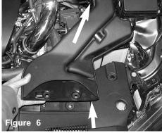
Pull up on the air scoop and pull forward in order to dislodge the air scoop from the air box cleaner.
