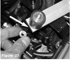
An m6 flange nut is used to fasten the vibra-mount to the end of the extension bracket.
