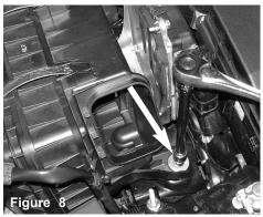
The m6 bolt is loosened from the base of the air box cleaner
