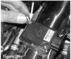
The stock screws are used to fasten the mass air flow sensor to the sensor adapter.
