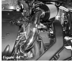
Periodically, check the fitment of both intake systems. Normal driving conditions may loosen nuts, bolts and clamps causing intakes to shift resulting in damage to automotive parts.
