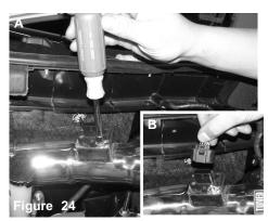
**Figure A:** Use a 7mm nut driver to tighten the 2 - 7mm bolts onto the MAF sensor. **Figure B:** Re-connect the MAF sensor onto the MAF sensor.
