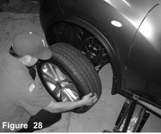
Re-install the wheel and make sure you torque the wheel to manufactures torque specs.
