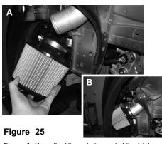
**Figure A:** Place the filter onto the end of the intake pipe located inside the bumper cover from the wheel well. **Figure B:** Filter on pipe
