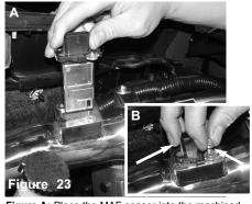
**Figure A:** Place the MAF sensor into the machined adapter on the Injen intale pipe. **Figure B:** Re-use the 2 -7mm bolts removed in figure 4
