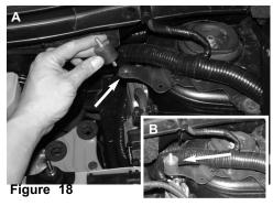
**Figure A:** Place 1 vibramount onto the factory air box housingbracket on the drivers side shock tower from figure 8. **Figure B:** Vibramount mounted onto shock tower bracket.
