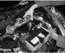
Lower the Injen intake tube into the engine bay and place the end of the tube into the bumpe cavity.
