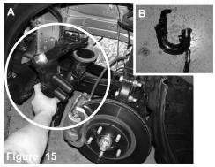
Figure A: You may now remove the resonator tube inside the bumper cavity. Figure B: Resonator tube removed
