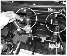
Figure A: Use a 8mm nut driver and loosen clamp on air duct to air box. Figure B: Loosen 10mm bolt on air box attached to bracket on shock tower.
