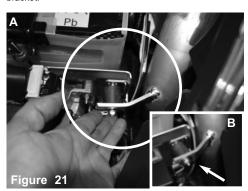
**Figure A:** Place a M6 nut and M6 washer on the vibramount on the second bracket is lined up. **Figure B:** Use a 10mm wrench and tighten the M6 nut
