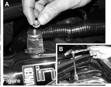
Figure A: Place a M6 nut and M6 washer onto the bracket located on the shock tower. Figure B: Use a 10mm socket and rachet and tighten the M6 nut
