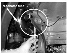
Once the wheel well cover is moved back, you can access the intake resonator tube inside the front bumper cavity. Remove the 10mm bolt attaching the resonator tube to the frame.
