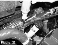
Adjust intake pipe for best fitment and then use a 8mm nut driver and tighten clamp on factory turbo intake duct tp the Injen intake pipe.
