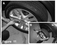
Figure A: Use a 21mm socket to remove the 5 wheel nuts. Figure B: Now remove the wheel
