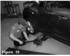
You will need to remove the driverside wheel. Use a jack to lift up the driverside wheel.
