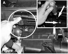
Figure A: Unplug the MAF sensor hraness from the MAF sensor. Figure B: Use a 7mm nut driver and remove the two 7mm bolts from the MAF sensor.
