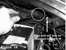
Remove the plastic clip underneath the drivers side headlight that is attached to the resonator tube.
