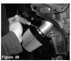
Tighten the filter clamp with a 8mm nut driver
