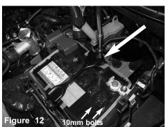
with 10mm socket and ratchet, loosen the battery brack- Now, carefully push the battery closer to the engine,
