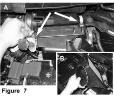
Figure A: Un-clip the two tabs on the top of the air box housing. Figure B: Remove the front of the air box housing
