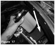
Install the filter and postion next to battery and fender.
