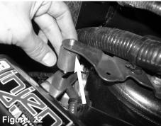
Tighten upwards and secure. Position the bracket on the intake tube.
