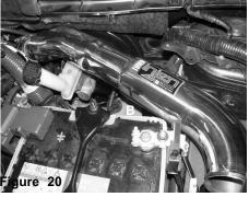
Position the intake tube and install into the hose from step 14. **Do not tighten.**
