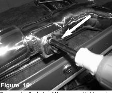
Secure using the factory M4 screws and tighten using 7mm nut driver.
