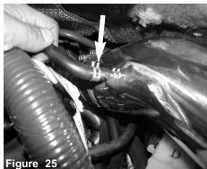
Install the vacuum line to the fitting on the intake tube.
