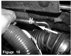
Remove the vacuum line from the fitting on the turbo auxillary hose. Pull back using pliers.
