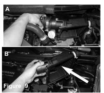
Figure A: Detach the air duct hose from the air box housing. Figure B: Remove the entire rear air box housing
