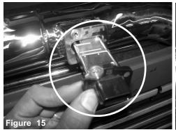
Install the MAF sensor into the new intake tube.
