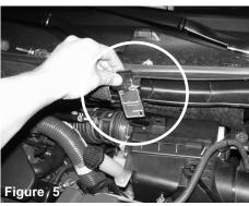
Pull the MAF sensor out of the factory air box hous-
