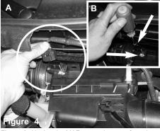
Figure A: Unplug the MAF sensor hraness from the MAF sensor. Figure B: Use a 7mm nut driver and remove the two 7mm bolts from the MAF sensor.
