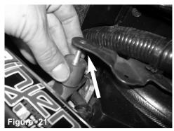
Install the vibra mount to the thredded fitting from under the bracket located on the strut tower.
