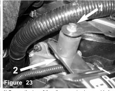
1) Secure the top of the vibra mount using provided M6 nut. 2) Secure the bottom of the vibra mount using provided M6 nut and washer.
