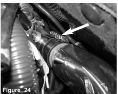
Tighten the clamps on the turbo using 8mm nut driver.
