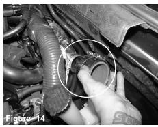
Install the 2" straight hose to the turbo using clamps provided. Tighten the clamp on the turbo only using 8mm nut driver.
