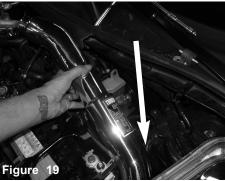
Install the intake tube. Note: position the filter side first into the vehicle first towards the filter, position so that the turbo side will slide into place.
