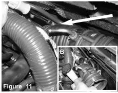
Figure A: With 8mm nut driver, loosen the clamp on the turbo. Figure B: Remove the stock turbo auxillary hose.
