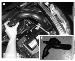
Figure A: Remove the air duct from behind the driverside headlight. Figure B: Air duct shown
