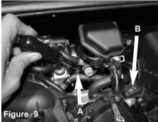
A) Loosen the clamp on the throttle body using 8mm nut driver. B) Remove the second bolt on air box.
