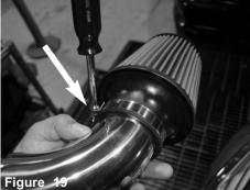
Install the filter to the tube and tighten. Tighten using 8mm nut driver.
