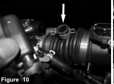
With pliers loosen the small clamp on crank case box located on the intake tube. pull back the box from the intake tube.
