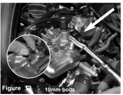
locate the bracket above on engine. loosen the bolt and Replace with provided M6 vibramount. remove the screw.
