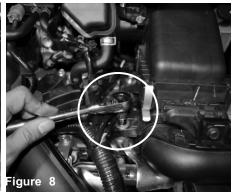
Loosen the bolt on the air box using 10mm socket and ratchet.
