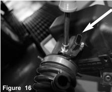
Loosen the 2 screws on the MAF sensor and remove. Remove the MAF sensor from the stock airbox. Save for later install.
