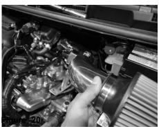
Install the intake tube. Position the intake tube to the hose and bracket to vibramount.
