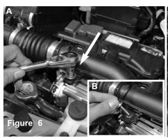
A) Loosen the bolt on ECU bracket using 10mm socket and ratchet. B) Remove the screw from assembly.
