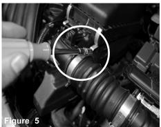
Loosen the clamps on the auxillary air line on air box using 8mm nut driver.
