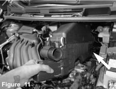
Pull back any lines that are attached to the air box assembly. Now lift up and remove the air box assembly out of vehicle.
