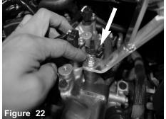
Secure the bracket using provided M6 nut and fender washer.
