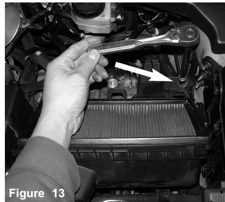
Figure 13 Then m6 bolt holding the air box to the fender well brace is loosened.
