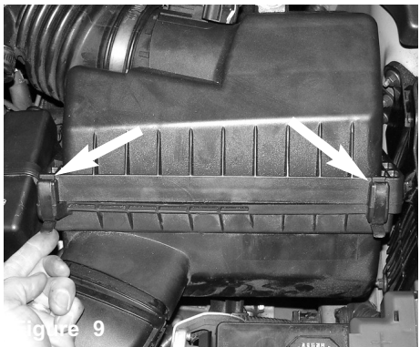
Figure 9 Unlatch the two metal clips shown above.
