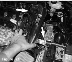
Install the intake system and position to the throttle body and the bracket to the vibra mount.
