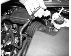
Disconnect the MAF sensor harness and pull line away from the air box.
