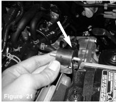
Next to battery locate the bracket and install the vibra mount to the fitting
