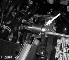
Secure the back of the vibra mount using m6 nut
