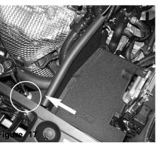
Secure and tighten the tab using provided M6 nut and fender washer.
