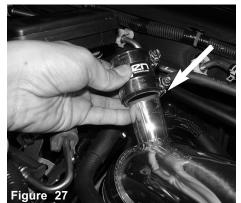
Install the 1.31 straight hose with clamps provided to the fitting on the intake tube.
