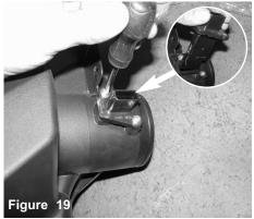
Loosen the 2 screws holding in the MAF sensor, and remove the sensor from air box.
