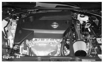
Once the intake and heat shield has been properly adjusted, continue to tighten all nuts, bolts and clamps. Re-install the engine cover and connect the battery terminals.
