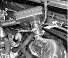
Now install the CCV box to the hose, *make sure the box is bottom-out and touching the fitting,* tighten clamps using 8mm nut driver.
