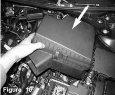
Now lift up and remove the air box from vehicle.
