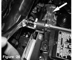
Now secure the bracket using provided fender washer and M6 nut. Secure and tighten using 10mm socket and ratchet.
