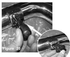
Now install the MAF sensor into the intake system. Secure and tighten using the factory 4mm screws
