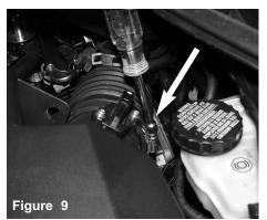
Loosen the clamp on the air box and pull back the intake tube.
