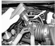
With pliers clamp off the CCV box from the intake tube.
