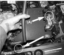
A)Now install the heat shield scoop and position the tab to the ECM thredded stud. B)Positon the other tab to thredded stud on radiator support.
