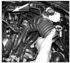
Lift up and remove the intake tube from the vehicle.
