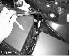
Loosen the bolt holding in the air box and remove.
