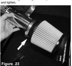
Install the air filter to the intake tube and tighten using 8mm nut driver.
