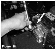
Secure and tighten the tab using factory nut from step 15.
