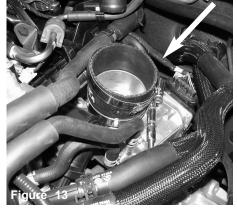
With clamps provided, install the 2-3/4" side to the step hose to the throttle body and tighten clamp using 8mm nut driver.
