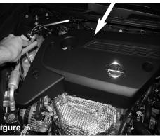
Loosen the 3 allen screws holding in the engine cover and remove.
