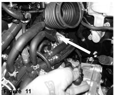
Now loosen the clamp on the throttle body using 8mm nut driver.
