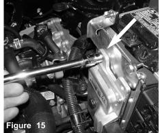
Next to battery, locate the nut holding in the computer ECM and loosen, save nut for later use.
