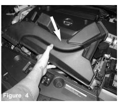
With 10mm wrench, loosen the 2 screws holding in the factory scoop and remove.
