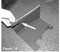
Now install the rubber trim to the top of the scoop heat shield.
