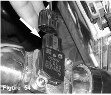
Press the electrical sensor harness over the mass air flow sensor until it snaps in place.
