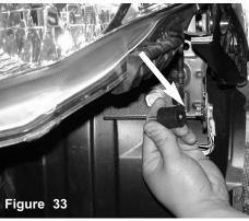
The male/female vibra-mount is aligned to the exposed bolt that holds down the grounding wires.
