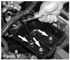
The three m10 bolts are loosened and removed from the lower air box as shown above.
