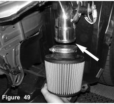
The new filter is aligned to the end of the intake and pressed in until its flush up against the filter stops.
