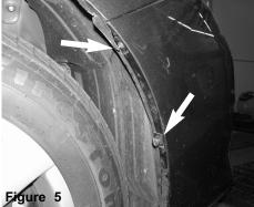
The two plastic clips are removed from side of the wheel well prior to pulling the bumper off.
