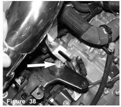
The primary intake lower bracket is aligned to the vibra-mount stud.
