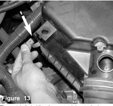
The metal clip holding the upper air box to the lower air box is unhooked from the top box.
