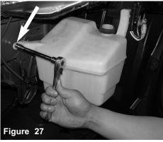
Loosen and remove the first m6 bolt from the reservoir bottle as shown above.
