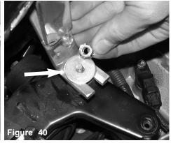
The m6 flange nut and washer is used to fasten the intake bracket to the vibra-mount stud.
