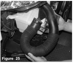
The lower air resonator duct is removed from the bottom of the air resonator air scoop.
