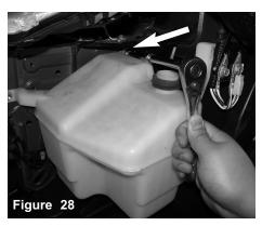
The last and final m6 bolt is removed from the reservoir bottle brace.
