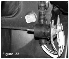
The male/female vibra-mount is now installed in the corner bumper cavity.
