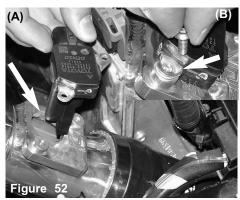
The mass air flow sensor is slowly lowered into the machined sensor adapter.(A), continue to use the m4 bolts in this kit to fasten the sensor in place (B).
