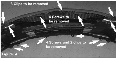
This is an illustration to show you how to remove the front bumper. Start by removing all plastic clips and screws as shown above, once all clips and screws have been removed continue to pull the front bumper off.
