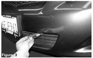
Prior to starting the installation, remove the 2 plastic clips inside of the grill.
