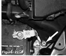
The m6 bolt is loosened and removed from the bottom of the resonator air scoop.
