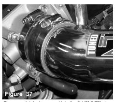
The upper intake is pressed into the 2 1/2"-2.75" stephose. A 8mm nut driver is used to semi-tighten the clamp.
