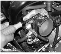
The 2 1/2"-2.75" step-hose is pressed over the throttle body, two power bands are placed over the over the hose. Tighten the clamp over the throttle body at this
