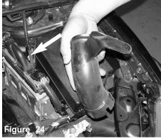
The resonator air scoop is now ready to be removed.
