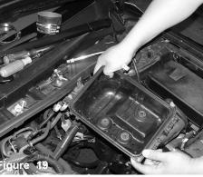
The lower air box cleaner is now pulled out from the engine compartment.
