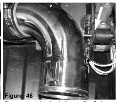
The secondary intake bracket is now sitting flush up against the vibra-mount. The m6 nut and washer are placed over the vibra-mount and intake bracket.
