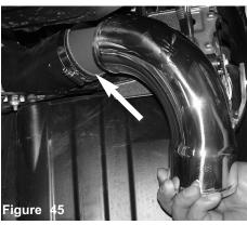
The secondary intake is pressed into the silicone hose and the intake bracket is aligned to the vibra-mount stud.
