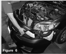
Once all plastic clips and screws have been removed, continue to pull off the bumper.
