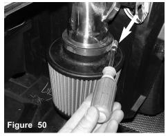
As soon as the filter stops have butted up against the secondary intake, continue to tighten the filter clamp with the put driver
