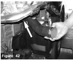
The 55 degree silicone hose is inserted through the driver side bumper cavity and into the engine compartment.
