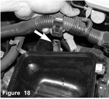
The lower harness brace is removed from the lower air box stand-off.
