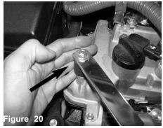
Secure the bracket using provided M6 nut and fender washer. Tighten using 10mm nut driver or wrench.
