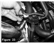
Secure the VSV to the crank case line using provided zip tie.
