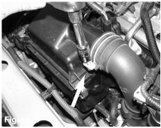
Loosen the clamp on the air box using 10mm nut driver or socket.
