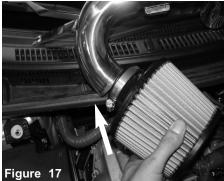
Install the filter to the intake tube. Tighten using 8mm nut driver.
