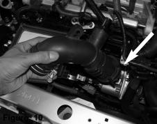
With pliers clip the clamp on the throttle body and remove the intake tube.
