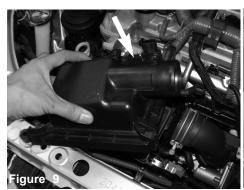
Disconnect the clips on the upper half of the air box and remove.
