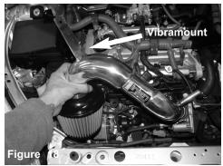
Install the intake tube into the vehicle and position the bracket to the vibramount and to the straight hose.
