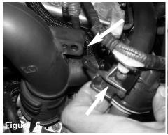
Pull back the VSV valve from the intake tube.
