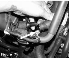
Pull back the crank case line from the intake tube fitting.
