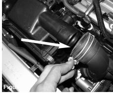
Pull back the intake tube from the upper part of the air box.
