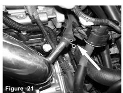
Connect the crank case line to the fitting and secure.
