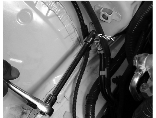
Use a 10mm socket and ratchet to remove the screw that secures the grounding wire to the fender well.
