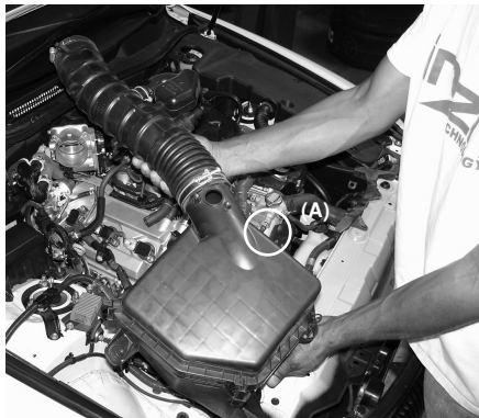
Lift and Pull the air box cleaner from the lower grommets. Before you pull the air box out, unclip sensor harness and remove from the side of the air box (A).
