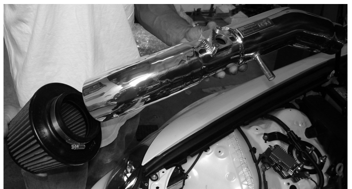
Slip the three inch filter over the end of the intake until it butts up against the filter stops. Once the filter has been firmly placed, continue to tighten the filter neck clamp.
