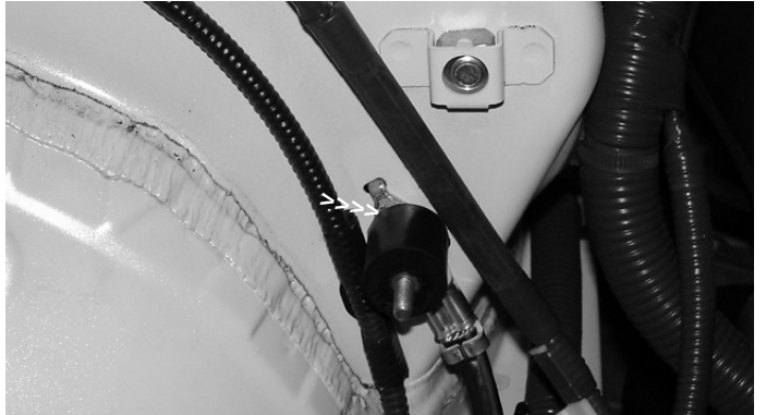
Screw vibra-mount firmly into the grounding wire pre-tapped hole until it bottoms out. Make sure the vibra-mount snug and tight over the grounding wires before moving on.
