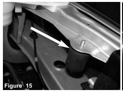
Secure and tighten the vibra mount.
