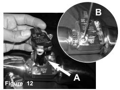
A) Now install the MAF sensor into the new injen intake tube. B) Secure using provided M4 screws and tighten using 2.5mm allen key.
