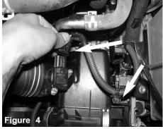
Disconnect the MAF sensor harness, pull harness away from the air box.
