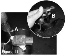
A) With philips screwdriver, loosen the 2 screws holding in the MAF sensor.
