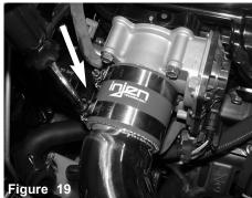
Position for the best fit, secure the bracket using provid- Position for best fit and tighten using 8mm nut driver.
