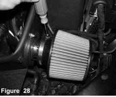
Now install the air filter and tighten using 8mm nut driver. Tighten all clamps using 8mm nut driver. Position for the best fit.
