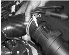
Pull back the stock intake tube away from the air box.
