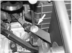
Tighten screw using 6mm allen key.
