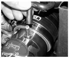
Now attach the vacuum line to the fitting on the intake tube and secure nice and tight.
