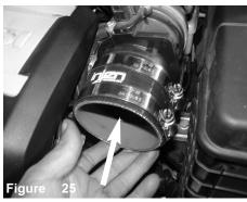
Install the 3-1/8" hose with clamps to the MAF sensor do not tighten.
