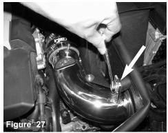
Now secure the bracket using provided washer and nut. Now position the intake tube for the best fit and tighten.
