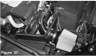
Align for best fit and tighten all clamps. Re-install the engine cover.
