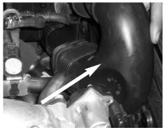
Carefully remove the plastic elbow connected to the air box and stock ram scoop.
