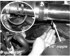
Now attach the 6mm vacuum hose to the welded 1/4" on the Injen intake tube. Picture shown vacuum line connected to intake tube.
