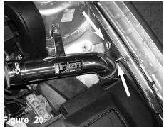
NOTE: Becareful with these two component in the engine bay when install the intake tube. Coming in contact with these can scratch the finish on the intake tube!
