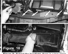
Figure A: Behind the headlight, there is a two piece plastic panel that you will remove four phillips screw from. Figure B: Once the four screws are removed, pull the entire two piece panel out.
