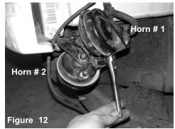
Note the original position of the two horns in the bumper Figure A: Unbolt 13mm nut on horn #2 and remount cavity. Use a 13mm socket and rachet to loosen nuts on horns and relocate horn #1 with horn #2.
