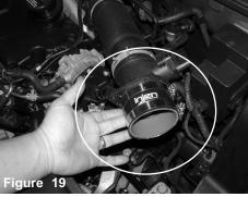
Place the 2.75" straight hose and two 040 clamps onto MAF sensor housing.
