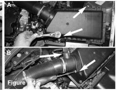
Figure A: use a 10mm socket and rachet and tighten the two 10mm bolts on the air box cleaner. Figure B:Use a T20 torx driver to loosen two torx screws from MAF sensor to air box cleaner
