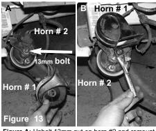
horn #1 onto horn #2. Figure B: Horn #1 is now mounted onto horn #2. This will allow room for placement of the Injen filter
