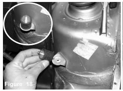
Mount the vibramount on to the factory bracket already mounted on the drivers side shock tower. Vibramount shown mounted on shocktower.
