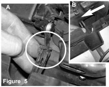
Figure A: On the back side of the grill is the unlocki ng clip for the hoodlatch. This clip need to be lifted in order to remove the latch from the hindge. Figure B: Hood latch is disconnected
