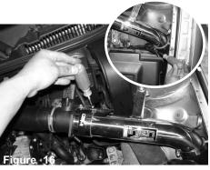
Once you have made final adjustments for the best fitment, use a 8mm nut driver and tighten the clamp on the MAF sensor hose and also the clamp on the TT silicon hose.
