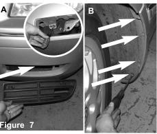
Figure A: Pull firmly on the lower outer grill to remove it to acess one torx bolt and repeat for the opposite side. Figure B: turn the steering inwards to access four t20 torx bolts on the plastic fender liner.
