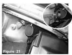
Position of the silicone TT hose in place. Place a 040 clamp onto the end of the silicone as seen in the photo
