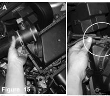
Figure A: PullI the MAF sensor housing out of the air box cleaner. Figure B: Unplug the vacuum line from the factory air box cleaner. This vacuum line is next to the opening where the MAF sensor use to go.
