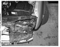
Figure A: Locate the two plastic rivets and then remove the the plastic frame behind the headlight. This frame will no longer be re-used in this installa-
