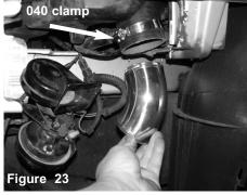
Place the smaller aluiminum intake tube into the silicone hose and make sure you add a 040 clamp onto the silicone intake tube.
