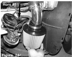
Place the 2.50" filter onto the 2.50" aluminum tube. adjust the pipe and filter for best possible fitment.. **NOTE:** horn #1 was relocated to make room for filter in figure 12
