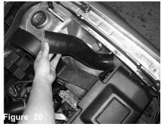
Place the silicone TT intake hose into the same path way the factory air duct once was. Make sure the bigger end of the silicone is on the top side.
