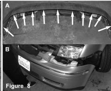
Figure A: There are 11 T20 torx bolts on the bottom side of the bumper that will need to be removed in order to remove the front bumper. Figure B: You may now remove the front bumper by pulling forward.
