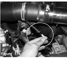
Place the 1 1/2" X1/4" aluminum coupler into the vacuum hose prevously removed from the air box assemble in figure 15
