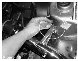
Align the intake bracket onto the vibramount and place a fender washer and M6 nut onto the bracket. Use a 10mm socket and rachet to tighten the nut to the vibramount.
