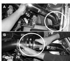
Figure A: Place the short end of the intake pipe and insert it into the TT silicone intake hose. Figure B: Now place the long end of the intake tube into the 2.75" straight hose previuosly installed in figure 19.
