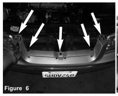
You now have access to the five torx bolts with the grill removed. Use a T25 torx driver to remove the five torx bolts
