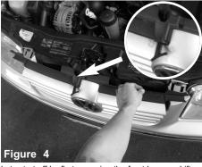
Lets start off by first removing the front bumper. Lift up on the front grill and pull towards you to unlatch the grill from the bumper. This will give you access to the hood latch that will need to be unhooked.
