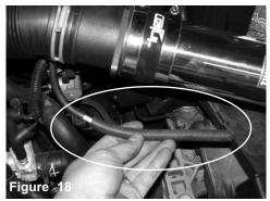
Connect the supplied 6" long 6mm vacuum hose to the 1/4 aluminum coupler from figure 17.
