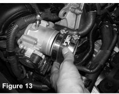
Place the 3.00" straight hose and 2 48 clamps onto the throttle body
