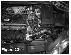
Check the alignment and fitment of the entire Injen intake. Once you have check for possible air leaks, rubbing or rattling, continue to tighten all nuts, bolts and clamps.
