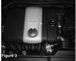
Picture of factory air intake system
