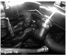
With light lubrication inside of the fittings on tube, secure and connect the crank case line and smog pump. Make sure you hear a click for it to be secured properly. *If not equipped, use provided vinyl plug.*
