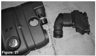
Optional engine cover/air box can be re-installed. Remove the snorkel ram air unit from the air box. Re-install to the engine.
