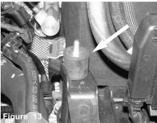
Secure and tighten the vibra mount.
