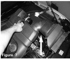
Lift up and remove the stock intake/engine cover from the vehicle. Pull up from each corner to pull from the engine grommets.
