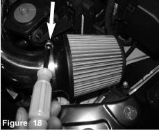
Install the air filter and tighten using 8mm nut driver.
