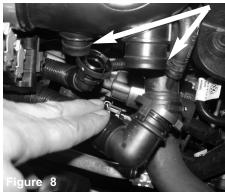
Disconnect the smog pump and crank case line from the stock intake tube.
