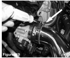
Position for best fit and clearance. Tighten the clamp using 8mm nut driver.
