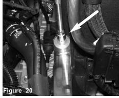
Now tighten the vibra mount using 10mm socket and ratchet.
