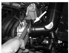
With pliers, loosen the clamp on the throttle body.
