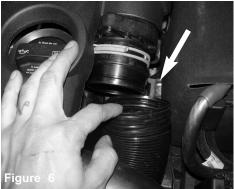
Pull back the intake tube from the air box.
