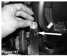
Secure the bracket using 10mm nut and fender washer.
