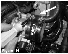
Install the 3" straight hose, with clamps and tighten on the throttle body.
