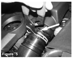
Loosen the flex clamp using pliers, slide over allowing you to pull back the intake tube.
