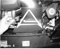
With T25 torx bit loosen the 2 screws holding in the factory scoop on the radiator support.
