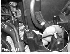
Loosen the 10mm screw on the bracket next to battery. Remove the screw.
