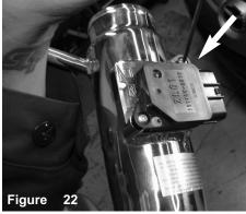
Secure the MAF sensor using provided M4 button head screws. Tighten using 2.5mm allen key.
