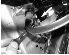
Tighten and secure the bracket using 10mm wrench or socket.
