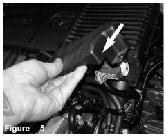
Loosen the clips holding in the Harness cover and remove.
