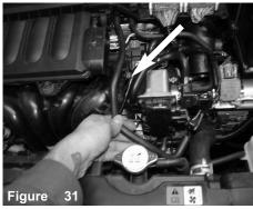
Route the vacuum line under the factory ram scoop.
