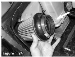
From under the vehicle, place the filter inside under the frame behind the splash guard.
