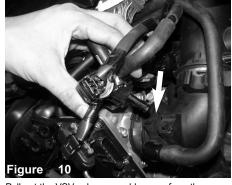
Pull out the VSV valve assembly away from the intake tube . Set aside for easier installation of the new intake system.
