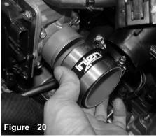
Attach the hose with clamps to the throttle body and tighten only on the throttle body.
