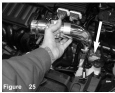
Install the intake tube into the vehicle and position the bracket to the vibra mount and to the throttle body.
