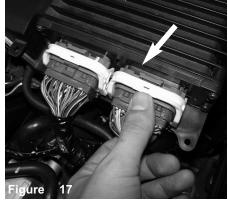
Before you continue, Re-connect the ECU and secure the AIR Box . This will still use the factory air box, allowing to cool the ECU.
