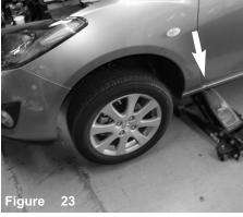
For easier installation, jack the driver side of vehicle just enough for you to get under the front of vehicle.
