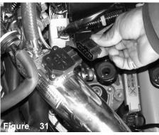
Press the electrical harness clip to the air mass sensor until it snaps in place.
