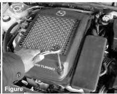
The two 6mm bolts are removed from the intercooler cover, this will give you easy access to the turbo inlet.
