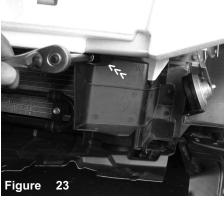
The third and final m6 bolt is removed from the splash guard.
