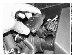
Carefully , remove the air mass sensor from the sensor Loosen the clamp that connects the air duct to the housing.
