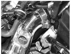
Once you have inserted the lower end into the bumper area, continue to press the upper intake into the step hose, semi-tighten the second power-band for now.
