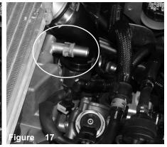
The green locking tab is also removed from the vacuum port.
