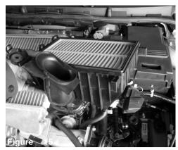
The lower air box cleaner is now pull out of the rubber plungers
