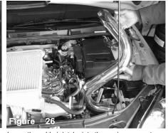
Lower the cold air intake into the engine compartment and into the bumper area.
