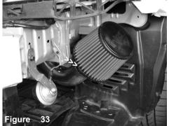
The tuned filter is now pressed over the end of the intake. Once the intake is butted up against the filter stop, continue to tighten the filter neck clamp.
