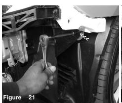
The first m6 bolt is removed from the splash guard.
