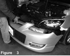
Remove 13-6mm bolts and 5 plastic clips in order to remove the front bumper.
