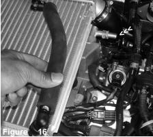
The upper breather hose is disconnected from the breather port as shown above. The stock hose is no longer used in this installation.
