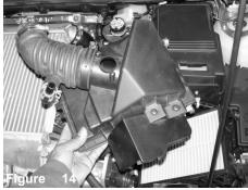
The top air box cleaner and air duct are now ready to be pulled out.
