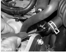
Use a small screw driver to depress the tabs on the hard line connector breather connector. This will allow you to separate the vacuum line from the plastic intake port.
