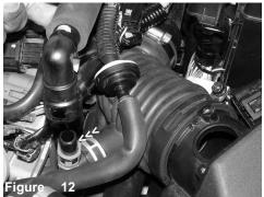
The 90 degree plastic elbow is now separated from the air duct breather port.
