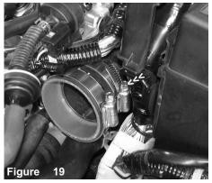
Press the step hose over the turbo inlet. Tighten the power-band on the turbo inlet side for now.
