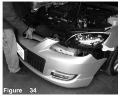
Once you have aligned and tightened all nuts, bolts and clamps, continue to install the front bumper to its original position.
