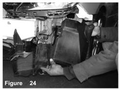
Once all bolts have been removed, continue to pull the splash guard out of the bumper section.
