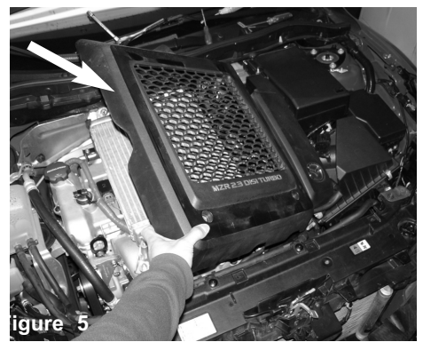
Figure 5 Once you have removed the m6 bolts, continue to remove the intercooler cover.
