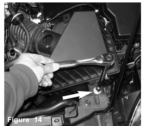
Figure 14 The air box bolt is loosened from the lower air box as shown above.
