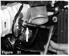
Tighten and secure the intake bracket using 10mm socket and ratchet.
