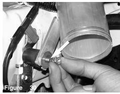
Secure lower intake tube to vibra mount using provided M6 fender washer and nut.
