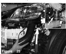
(A) Install silicon intake hose through bottom of headlight.
