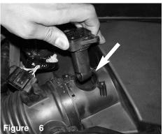
Carefully remove the electrical MAF sensor from sensor housing.
