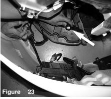
Installing the cold air intake: Remove 13 - 6mm bolts, If equipped with fog lights, disconnect light harness.
