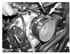
Press the silicon hose with clamps over the throttle body hose. Tighten the clamp over throttle body only using 8mm nut nut driver.
