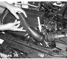
Carefully remove the plastic air intake duct.
