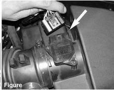
Disconnect the electrical MAF sensor harness.
