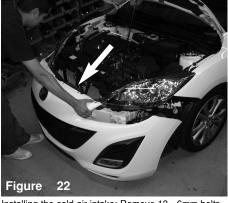
Installing the cold air intake: Hemove 13 - 6mm bolts, 5 plastic clips and 2 phillips screws in order to remove the front bumper.
