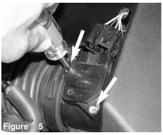
With phillips screwdriver, loosen the 2 screws holding in MAF sensor.
