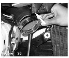
place clamp over the silicon hose as shown above but do not tighten.
