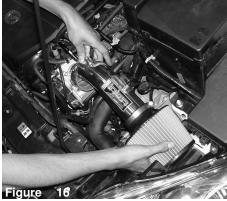
Carefully, lower the entire assembled intake system into position. Align the intake bracket to the vibramount stud.
