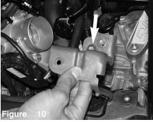
The air box bracket is removed from itscurrent location, this bracket will no longer be used with for the intake.
