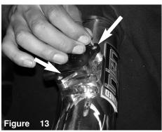
Insert the electrical MAF sensor to intake tube. Secure the sensor by using the provided M4 button head screws.
