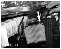
Press the tuned air filter over the lower intake tube. Once the intake is butted up against the filter stop, continue to tighten the filter neck clamp using 8mm nut driver.
