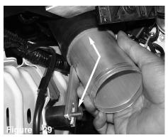
Align and position lower intake tube to silicon elbow and vibra mount.
