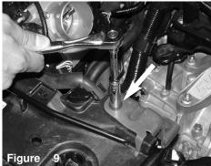
Loosen the 10mm bolt that fastens the air box bracket over the radiator support.
