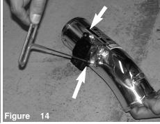
Tighten MAF sensor using 2.5mm allen key.
