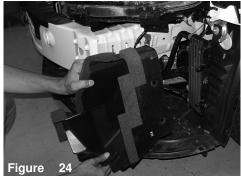
Remove CVT cooler splash guard. Loosen the 3 plastic push clips using phillips screwdriver.
