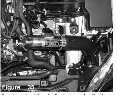
Align the entire intake for the best possible fit. Once you have rechecked and cleared the intake from all moving parts, continue to tighten all nuts, bolts and clamps.
