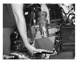
Remove the entire air intake box assembly from the engine compartment.
