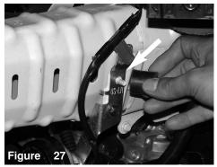
Attach female side of vibra mount to M6 stud on horn bracket
