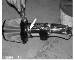
Press the tuned air filter over the intake tube, tighten the clamp on the filter using an 8mm nut driver.
