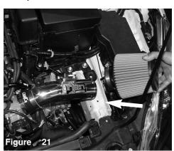
Loosen clamp and remove the tuned air filter.
