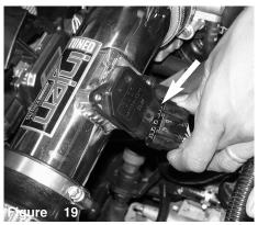
Re-connect electrical MAF sensor harness.
