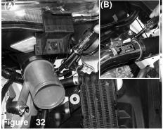
Tighten all clamps on lower intake located on the silicon intake hose (A) Now tighten the clamp on the upper silicone intake using an 8mm nut driver.
