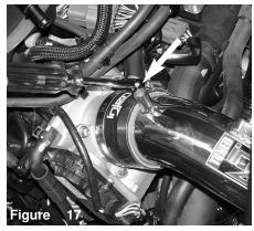
Once you have aligned the intake bracket to the vibra-mount stud, continue to tighten the clamps using using an 8mm nut driver.
