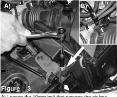
A) Loosen the 10mm bolt that secures the air box cleaner. B) Dislodge the crank case hard line from stock vacuum port on the air intake duct.
