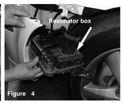
When all bolts have been removed the detach the resonator box from the frame.
