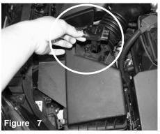
Pull the MAF sensor out of the factory air box
