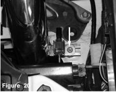
Place a M6 nut and fender washer onto the intake bracket and tighten the nut down to secure the intake to the switching valve. No vauum line will be connected the vibramount
