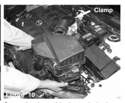
Once you have loosened the clamp on the throttlebody, you may now pull up on the air box assembly dislodging the air box from the air box bracket grommets
