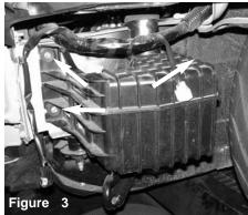
Once the bumper has been pulled back, continue to remove the three bolts holding the air resonator box to the frame.
