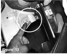
Remove the 10mm bolt on the grounding junction. This grounding junction will be relocated in figure 14
