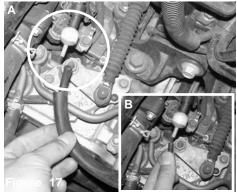
Figure A: Remove the 4mm vacuum line connected to Lower the intake into the engine compartment, place the half green check valve removed from the factory air the pipe into the 45 degree hose and align the intake box assembly in figure 8. Figure B: Place the 5mm vacuum cap over the check valve
