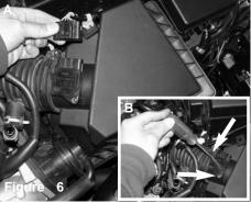
**Figure A:** Unclip the MAF sensor harness off the MAF sensor. **Figure B:** Use a phillips screw driver and remove the two screws on the MAF sensor
