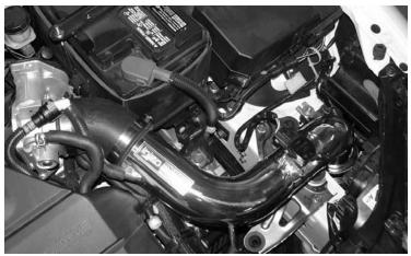
Congratulations! You have just completed the installation of this cold air intake system. Periodically, check the fitment of this intake system to avoid shifting of the intake that may damage the intake from rubbing and banging to other metal parts.
