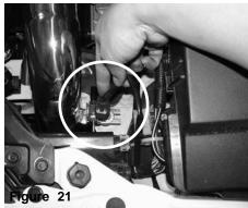
Reconnect the green VAD switching valve harness to to the switching valve. The ECM just needs to see it is functioning
