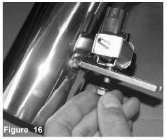
With the filter end of the intake facing down, place the solenoid on top of the intake bracket and use the same nut to fasten the solenoid to the intake bracket.
