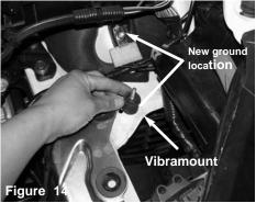
Place the vibramount on the old location of the grounding junction. The grounding junction will be relocated on the factory threaded stud on the relay box bracket
