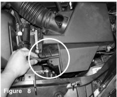
Disconnect the 5mm vacuum line from the fron of the air box assembly.
