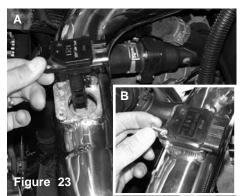
Figure A: Place the MAF sensor onto the machined welded flange. Figure B: Place 2-M4 button head screws onto the MAF sensor
