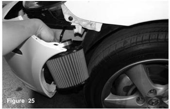
Align the filter to the end of the intake (A). Press the filter over the intake end until the intake has butted up against the filter stops (B) Tighten the clamp on the filter neck to prevent the filter from falling off.
