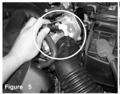
Pull the breather line out of the factory air duct hose
