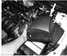
Disconnect the crank case line from the engine. Unclip the upper half of the air box and remove the assembly.
