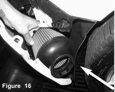
Now install filter into the bumper compartment.
