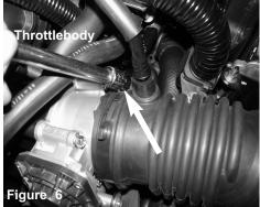
Loosen the clamp on the throttle body using 10mm socket and ratchet.
