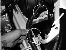
locate the harness that is behind the head light. pull the clips away from the frame allowing more room for clearance for the intake install.
