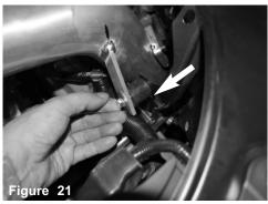
Secure the bracket to the vibramount using provided m6 nut and fender washer. Do not tighten.
