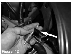
Locate the tab on vehicle frame behind the headlight.
