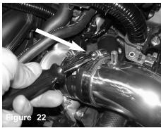
Position the intake for the best fit. Tighten the clamp using 8mm nut driver.
