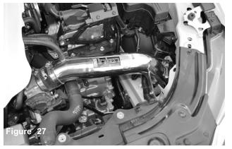
Check the entire system for the best possible fit. Once you have checked the entire system for leaks, rubbing or rattling, continue to tighten all nuts, bolts and clamps. Reconnect the negative battery terminal prior to starting the engine.
