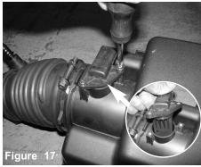
Loosen the screws holding in the MAF sensor. Remove the MAF sensor.
