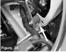
Secure and tighten the bracket using a 10mm socket or wrench.
