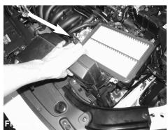
Now lift up and remove the bottom half of the air box.
