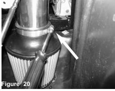
Now attach air filter to the intake tube and tighten using 8mm nut driver.
