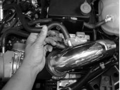
Take the stock crankcase breather line and press it over the 1/2" port on the intake, use the stock clamp to keep the line from slipping off.
