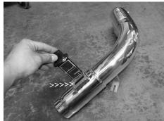
Carefully place the mass air sensor into the calibrated machined adapter.
