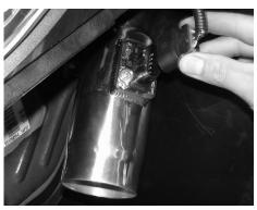
Once the intake has been carefully aligned, take the ECU harness and press it over the mass air sensor. You will hear a short snap when the harness has sensor have been properly connected.
