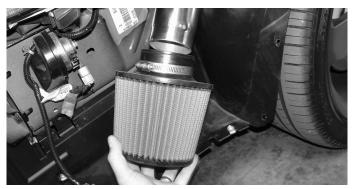
Press the Injen filter over the end of the intake as shown in this picture. Once the filter has been pressed in place continue to tighten the filter neck clamp.
