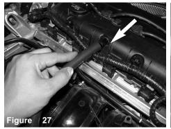
Install provided 10mm hose to crank case on engine
