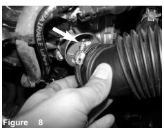
Pull back intake tube from throttle body.
