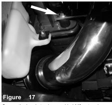
Secure the bracket using provided M8 nut and washer.
