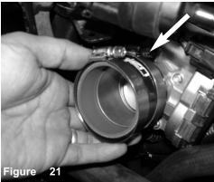
Install the 2-1/4" straight hose with clamps provided to throttle body and tighten on throttle body only.
