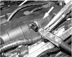
Disconnect the electrical MAF sensor harness.
