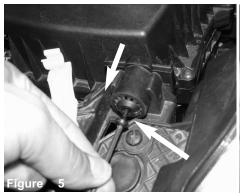
With 4mm allen key, loosen the screw holding in air box grommet and remove.
