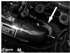
Position best possible fit and tighten remaining clamps using 8mm nut driver.
