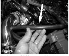
Attach new provided 8mm hose to intake tube and plastic fitting.
