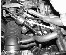
With flat head screwdriver, loosen the clamp on throttle body.
