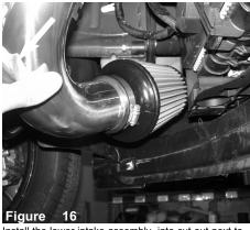
Install the lower intake assembly into cut out next to washer resovoir and radiator. Position the bracket on intake tube to vibra mount.
