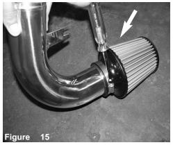
Attach the air filter to lower intake assembly and tighten.
