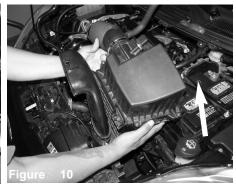
Carefully lift and pull out air box.
