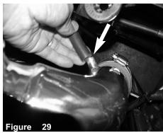
Connect the new hose to the fitting on the tube,
