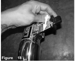
Install the MAF sensor into new intake tube.
