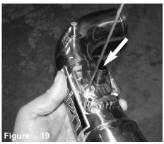
Secure and tighten the MAF sensor using provided M4 button head screws using 2.5mm allen key.
