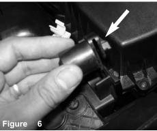
Carefully remove the grommet from air box.
