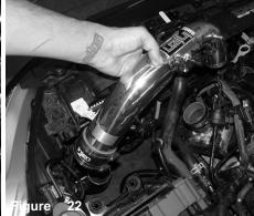
Install upper intake tube assembly and position to lower intake tube and throttle body. Connect the 2 intake tubes together.
