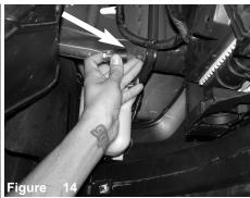
For easier installation, you can carefuly lift front of vehicle. From under neath vehicle or from up top, attach M8 male/female vibra mount to stud on frame next to washer resovoir and secure.
