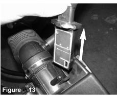
With T20 torx bit, loosen and remove the 2 screws hold- Carefully remove MAF sensor from air box.
