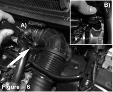
A) Loosen the clamp on the intake tube. B) Locate the vacuum line fitting on the engine, disconnect fitting. Pull back line this will allow for easy removal and installation of intake system.
