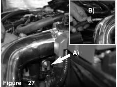
A) Secure the bracket using provided M6 nut and fender washer. Do not tighten.
