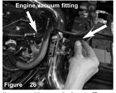
Now re-connect the vacuum line from step 6B. Connect the MAF sensor harness.
