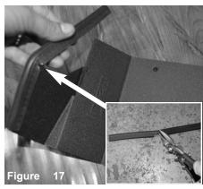
Install the bulb trim to the top of the heatshield. Cut the corner and notch a V for a clean cut and bend.
