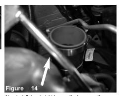
Now install the straight hose with clamps on the turbo. Tighten the clamp on the turbo side only.
