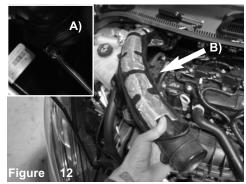
A) Locate the turbo and loosen the clamp on turbo holding in the intake tube.
