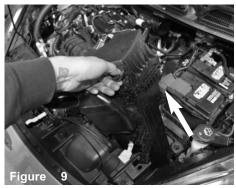
Now lift up and remove the stock air box out of vehicle.
