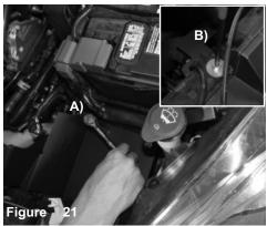
A) Tighten the 2 bolts using 13mm socket and wrench. B) Secure M6 allen screw using 5mm allen key.
