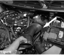
Remove the intake tube from vehicle.
