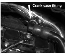
Connect the Crank case line to the fitting on intake tube. Use some lubrication inside the fitting for easier installation. Make sure you hear a click.
