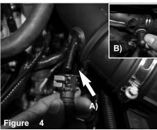
A) Disconnect the vacuum line from the fitting on stock intake tube.
