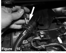
Locate the screw/engine cover fitting. This holds in the factory intake tube to turbo. Save for later install  $% \left( x\right) =\left( x\right) \left( x\right)$ for the engine cover.
