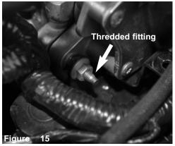
Locate the M6 thredded fitting on side of engine. See figure 6B for the location right under the vacuum fitting.
