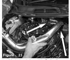
Install the intake tube into vehicle. Position like above image to install. Slowly rotate tube to the hose on turbo.
