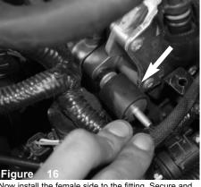
Now install the female side to the fitting. Secure and tighten.
