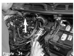
Now install the intake tube to the hose on turbo and position the bracket to the vibramount from steps 15/16. Do not tighten.
