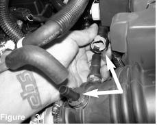
Disconnect the crank case line, also pull back the vacuum line from fitting.
