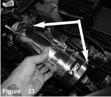
Install the upper intake tube into and position to the lower intake and the throttle body.
