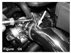
Tighten the clamps on throttle body using 8mm nut driver.
