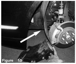
Remove the push clips from the splash guard and pull back, this will allow for removal of factory resonator.
