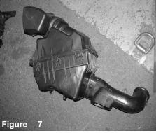
Remove the complete stock airbox as shown in above image.
