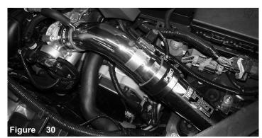
If vehicle was jacked up, lower vehicle. Connect battery terminals. For short ram install, remove the lower intake assembly and place filter on upper intake tube assembly. See figure 31.
