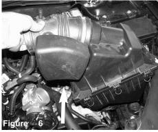
Carefully lift up and remove the stock intake system out of vehicle.
