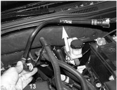
Remove the crank case line from the engine compartment.
