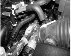
Loosen the clamp on the throttle body using 8mm nut
