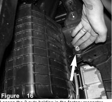
Loosen the 3 nuts holding in the factory resonator using 10mm socket or wrench.
