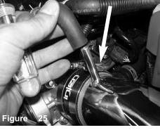
Reconnect the vacuum line to the fitting on the intake tube.
