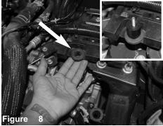
Make sure the factory air box grommet is still in position. Install the provided M6 stand off stud to the grommet.
