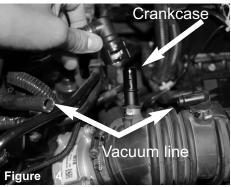
Pull back the vacuum line. Disconnect the crankcase line.
