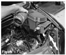
Lift up and remove the air box assembly from the vehicle, make sure the fitting pop out from grommets under neath air box.
