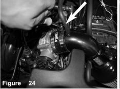
Position for the best fit, tighten the clamp on intake tube using 8mm nut driver.
