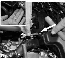
With socket cap screw and m6 nut, tighten the scoop to heat shield.
