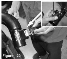
Now install the MAF sensor into the intake tube. Secure and tighten using provided M4 button head screws.
