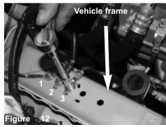
Loosen the 3rd ground strap. Save bolt for later install.
