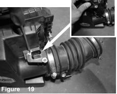
With T25 torx bit, loosen the 2 screws holding in the MAF sensor. Remove the MAF sensor.
