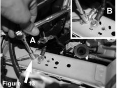
A) Loosen the 1st ground strap.B) Now flip the connection fitting over upside down and secure to the first ground strap. Tighten using 8mm socket.
