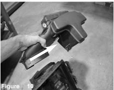
Carefully remove the scoop from the air box.
