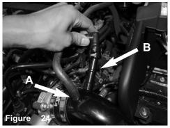
A) Now attach the vacuum line to the 3/8" fitting on intake tube. B) Connect the crank case line to the machined fitting on intake tube. Page 3 of Part# SP9062
