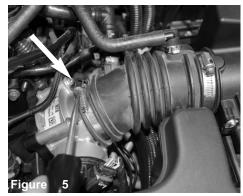
Loosen the clamp on the throttle body.
