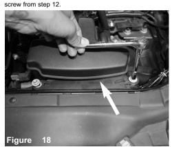
Now secure the front of the scoop using the factory screws.
