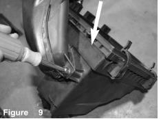
With 8mm nut driver, loosen the 2 screws holding in the scoop.
