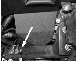
Now secure the stand off stud using provided m6 nut and fender washer. Secure the heatshield using factory
