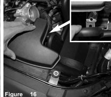
Install the air scoop. Secure the back of the heatshield to the scoop.
