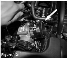
Install the straight hose with clamps to the throttle body. Tighten the clamp on throttle body only.
