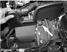
Install the provided rubber trim to the top of the heatshield, notch in corners with knife or scissors for cleaner installation.Install the provided m6 stand off stud to factory grommet air box position.
