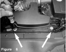
Loosen the 2 bolts holding in the OEM ram scoop using 8mm nut driver. Pull back the hose from the throttle body.
