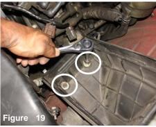
once you have pulled off the top air box lid, continue to loosen and remove the two m6 bolts located on the bottom of the air box.
