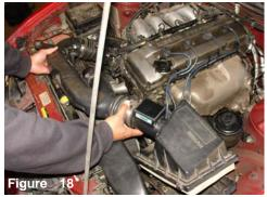
Here is another view of the air box cleaner and air intake pipe being pulled out of the engine compartment. Notice that the air filter panel is also pulled out.
