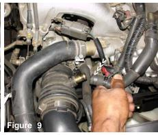
Once you have removed the tension clamp, continue to disconnect the CVC breather hose from the air intake port.
