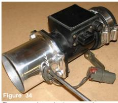
The screws are fastened to the sensor pad.
