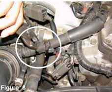
Using a set of pliers, depress the tension clamp on the hose and pull the clamp away from the air intake port
