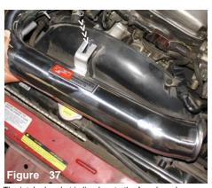
The intake bracket is lined up to the fan shroud threaded hole.
