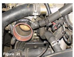
Press the 2 3/4" straight hose over the throttle body, use two power-bands on the hose but only tighten the clamp on the throttle body for now.
