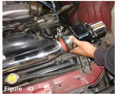
The assembled mass air flow sensor is now pressed over the end of the intake, Semi-tighten the powerband once the air sensor has been adjusted.
