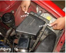
Disconnect the two clamps connecting the top air box to the lower air box.
