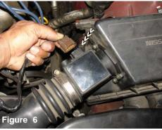
Depress the upper tab on the harness clip and disconnect the harness clip from the mass air flow sensor
