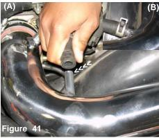
The air bypass line is now pressed over the large intake port by the fan shroud (A). The stock clamps are used to secure the hose over the intake port (B).
