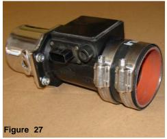
The mass air flow sensor, filter flange, straight hose and power-bands are now assembled.
