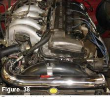
The air intake is in place and ready to secured.
