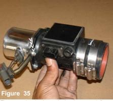
The sensor bracket is attached to the mass air flow sensor bolt.
