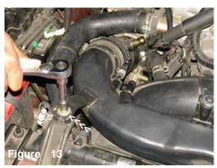
Loosen the m6 bolt from the radiator bracket as shown above.
