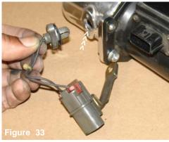
The sensor is now inserted into the sensor pad located on the filter flange. The stock screws are used to fasten the air temperature sensor to the sensor pad.
