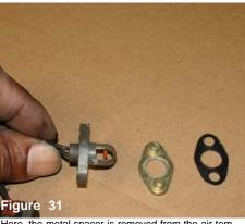
Here, the metal spacer is removed from the air temperature sensor along with the gasket. The gasket is replaced and used in the application.
