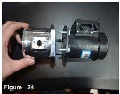
Take the sensor flange and 4- m6 x 25mm bolts and butt it up to the mass air flow sensor.
