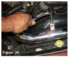
The stock bolt is used to fasten the intake to the fan shroud
