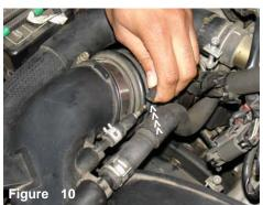
Disconnect the vacuum switching valve line from the air intake port coupler.
