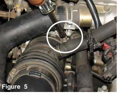
Loosen the clamp on the throttle body intake duct.
