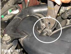
Depress the tension clamp on the air bypass line and pull the tension clamp away from the air intake port as intake port. shown above.
