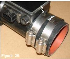
Press the 2 3/4" straight hose over the mass air flow sensor, use two power-bands on the straight hose. Tighten the clamp located on the mass air flow sensor.
