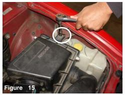
Loosen and remove the m6 bolt holding the top air box to the fender well brace.
