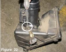
Remove the first bolt from the mass air flow sensor housing that holds the harness bracket and harness clip
