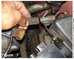
Depress the tab on the harness clip connected to the air temperature sensor and remove the harness clip.
