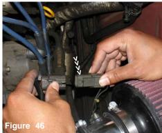
Insert the sensor connector into the air temperature sensor clip as shown above.
