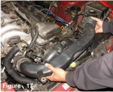
Once all clamps and bolts have been removed, continue to pull the air intake out along with the top air box cleaner.
