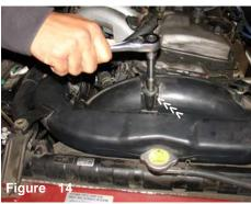
Remove the bolt located over the fan shroud. This will allow you to remove the air intake.
