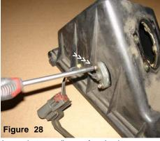
Loosen the two small screws from the air temperature sensor that fastens it to the upper air box cleaner.
