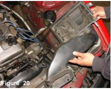
Now that the four bolts have been remove, continue to pull the front air scoop and lower air box cleaner for the engine compartment.
