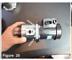
Take the 4- m6 flange nuts and fasten the nuts to the m6 bolts on the sensor flange. Secure them tight so that the flange is secure.
