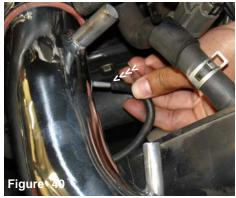
The vacuum switching valve line is pressed over the 5mm vacuum port.
