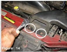
Loosen and remove the two m6 bolts holding the air scoop over the cross member.
