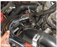
Take the Injen intake and lower it into the engine compartment, over the fan shroud. The intake is pressed into throttle body hose.
