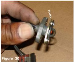
Use a screw driver to pry lose the metal spacer that is glued to the air temperature sensor.
