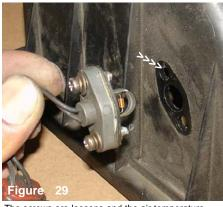
The screws are loosens and the air temperature sensor is removed from the air box top.
