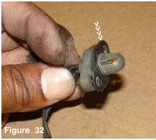
The gasket is placed on the air temperature sensor as shown above.
