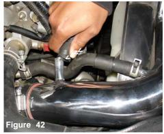
The CVC line is pressed over the large intake port by the throttle body. Use the stock clamps to secure the hose to the intake port.
