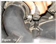
The air bypass line is disconnected from the air intake port.
