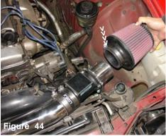
Take the filter and press it over the intake end. Once the intake is butted up against the filter stops, continue to tighten the filter clamp.
