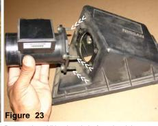
Remove the additional m6 bolts from the air box cleaner top and remove the mass air flow sensor as shown above.
