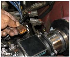
Press the electrical sensor harness clip over the sensor until it snaps in place.
