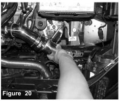
Place the Long Injen intake pipe through the opening under the drivers side headlight.
