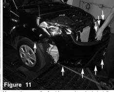
You must remove the front bumper in order to install this intake system. Remove all the screws and plastic retaining clips indicated in the photo and then pull the front bumper off.
