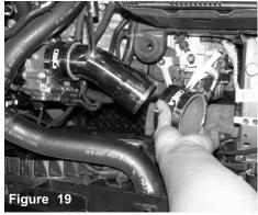
Place the 2.75" hose and two #48 clamps onto the 2.75" end of the intake pipe
