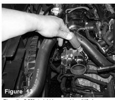
Place the 2.50" straight hose and two #40 clamps onto the throttle body and only secure the clamp on the throttle body side only for now.
