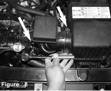
Use a 10mm socket and rachet and loosen the clamp on the throttle body side and air box side of the air duct hose.
