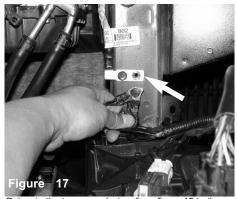
Relocate the two ground wires from figure 15 to the transmission ground wire. Reuse the 10mm bolt and secure the ground wires to the chassis. Relocating the ground wire will allow slack in the main wire harness.
