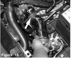
Place the short injen intake pipe with the 2.50" end onto the throttle body hose
