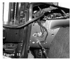
Locate the two ground wires under the headlight on on the drivers side wheel well. Unbolt the two 10mm bolts securing the ground wires to the chassis.
