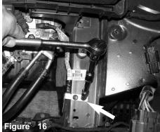
Remove the right bolt on the transmission ground wire located in the engine bay. The two ground wires from figure 15 will be relocated to this grounding point
