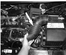
disconnect the air duct from the throttle body and air box and remove the air duct hose
