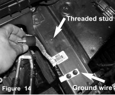
Place the Injen male/female vibramount onto the threaded stud on the chassis where the stock air box assembly once was. You can use the transmission ground strap for reference
