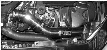
Your intake installation is now complete. Go over all your clamps and fittings to make sure they are snug. Check the clearance on the pipe and make sure it does not make contact with any components in the engine bay.
