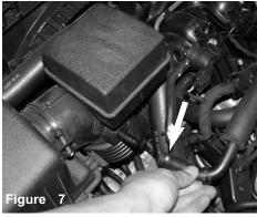
Disconnect the crank case vent tube from the air box air duct hose.
