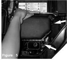
Use a 3/8 -10mm socket with extension and rachet and loosen the two 10mm bolt on the air box assembly.
