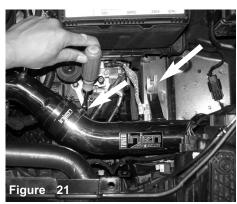
Position the intake pipe for best possible fitment. Align the intake bracket to the vibra mount from figure 14. Now secure the #48 clamp on the 2.75" hose securing the two pipes together.
