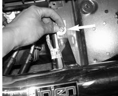
Place the supplied M6 nut and fender washer onto the threaded stud on the vibra mount. You may down tighten the M6 nut to secure the intake bracket to the vibra mount
